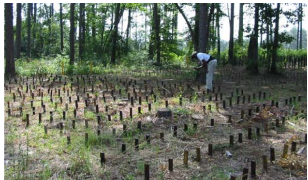
Field stake testing is extremely important when evaluating new wood treatments.
