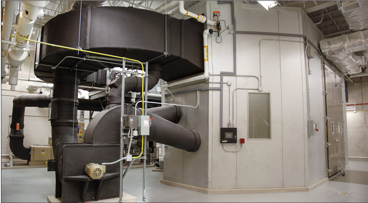
Figure 2—Chamber for Analytic Research on Wall Assemblies exposed to Simulated weather (CARWASH) facility [credit: Steve Schmieding].
