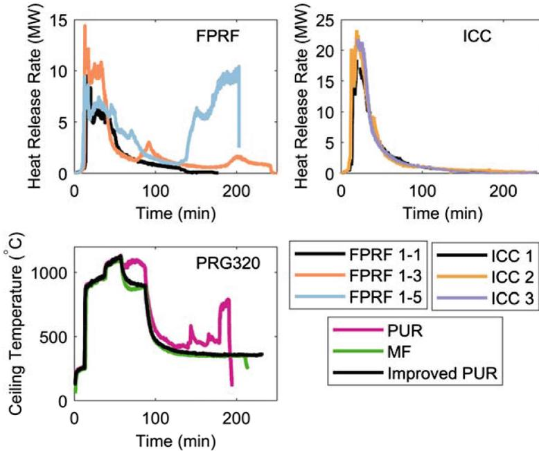
**Fig. 1.** Relevant test data from the three large scale test series discussed in the paper. (Data replotted from [7–9]).
