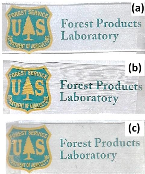
Figure 3: Photograph of films: a) PLA with freeze-dried CNCs; b) PLA wet-blended control (No CNCs or additives); c) wet-compounded PLA with 1% DTAC-CNCs and 10% PVAc
