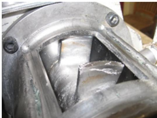
Figure 1: Thermokinetic mixer shown with open chamber
