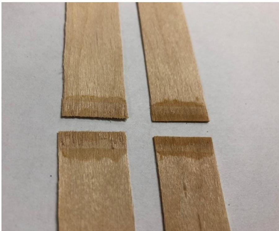
**Figure 4: Analysis of failed sample. Adhesion failure on the left and cohesive failure on the right. Please click here to view a larger version of this figure.**
