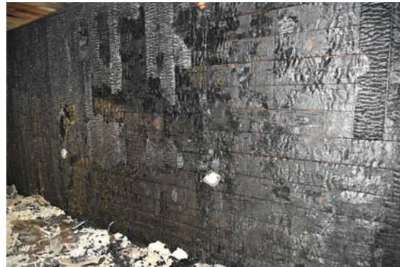
**Figure 2:** Full scale compartment fire test on CLT building conducted in 2017 by FPL (top) and example of a delaminated surface (bottom)
