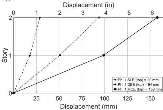
Figure 6: Displacement profile for SLE, DBE, and MCE
