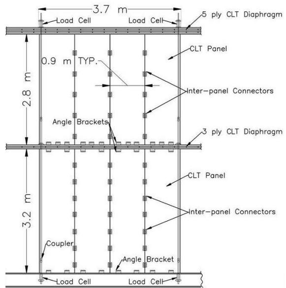
Figure 3: Shear wall stack layout
