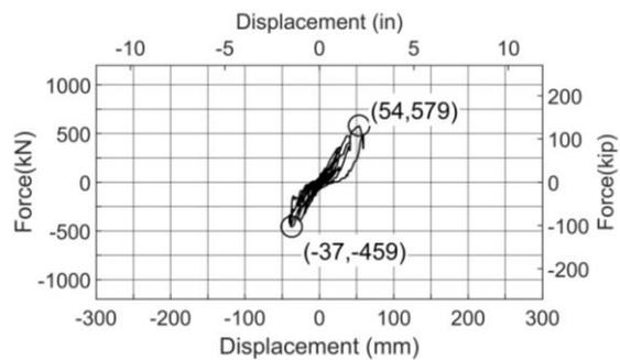
Figure 10: Second story shear versus story displacement
