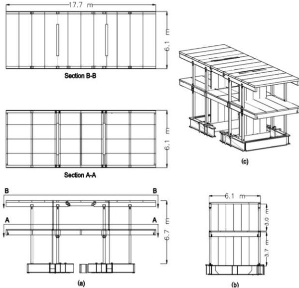
Figure 1: Elevation, plan, and isometric views of test specimen
