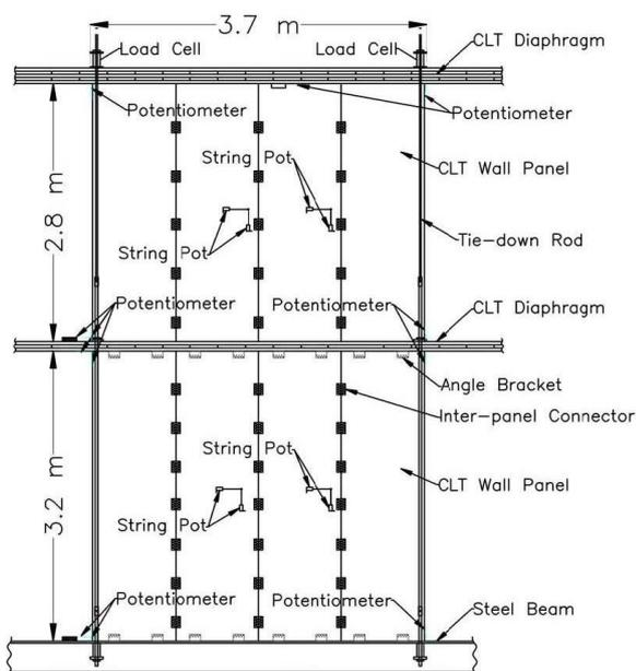
Figure 4: Shear wall instrumentation deployment
