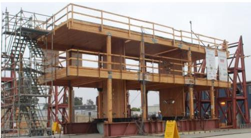
Figure 2: Two-story test specimen on shake table
