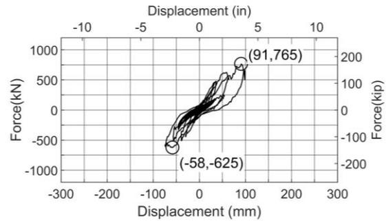
Figure 9: First story shear versus story displacement
