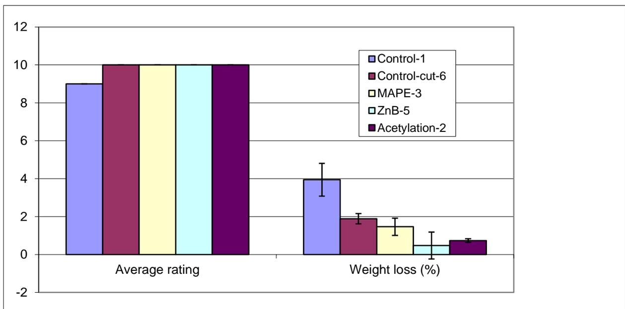
Figure 4: Field test results after 30 months exposure to *C. curvignathus*. (Not shown: Solid wood pine specimens had an average rating of  $0.9\pm 1.91$ , and  $92.2\pm 16.8\%$  weight loss.)
