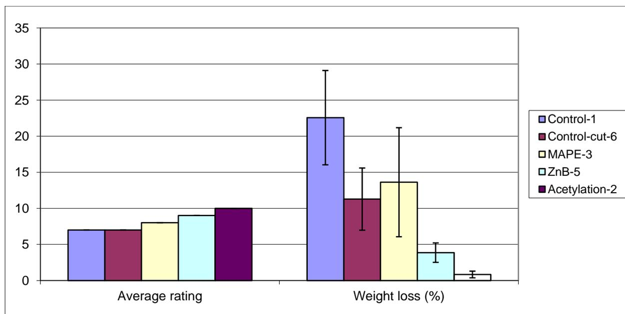
Figure 5. Field test results after 30 months exposure to *M. gilvus*. (Not shown: All solid wood pine specimens had average rating of 0 and 100% weight loss after 30 months.)
