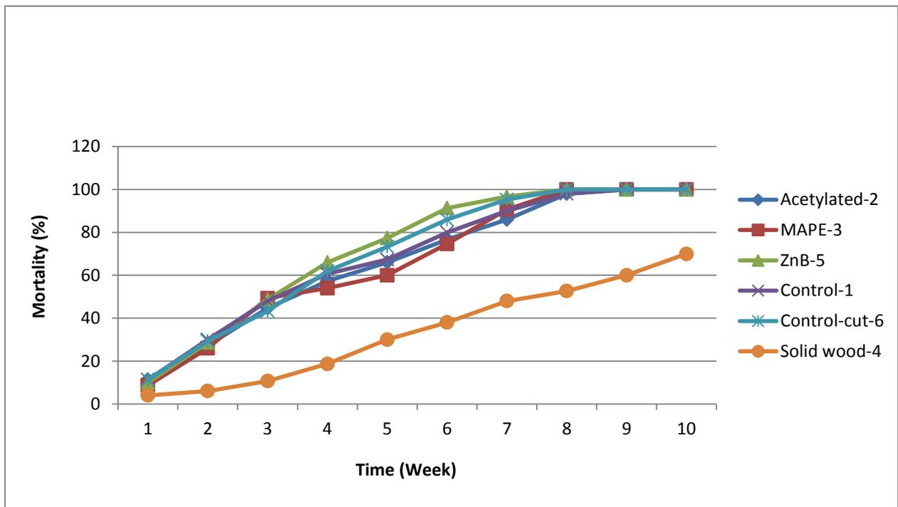
Figure 1: Laboratory dry wood termite test results after 10 weeks exposure to *C. cinocephalus*.
