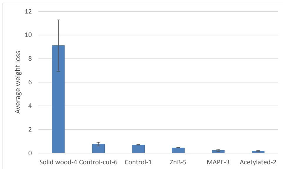
Figure 2: Average weight loss after the 10 week dry wood laboratory termite test.
