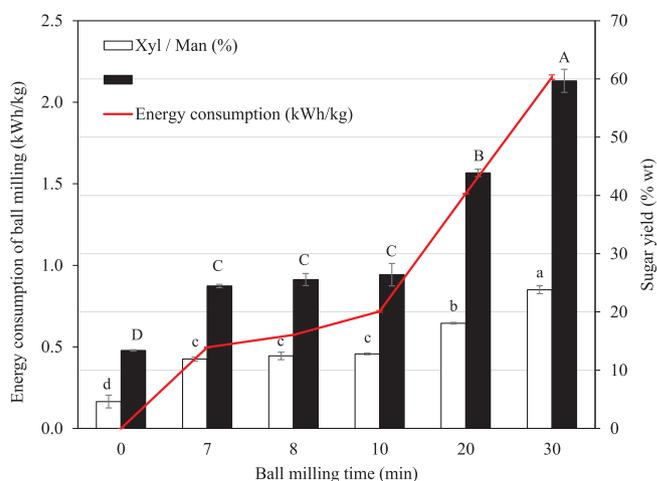
Fig. 3. Sugar yield of Douglas-fir forest residuals at various ball milling time with different energy consumption. Different letter above the bars indicate values significantly differs at  $p < .05$  level. Capital letter (A, B, C, and D) indicates compared means of glucose yields (% wt) and small letter (a, b, c, and d) indicates compared means of Xyl/Man (% wt).
