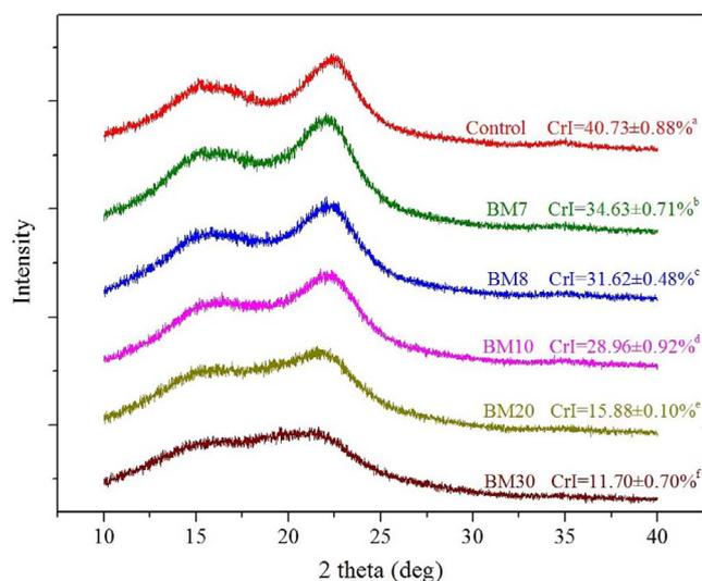
Fig. 2. Effect of ball milling time on X-ray diffraction of wood residuals. Different alphabet superscripts indicates that means of crystallinity index were significantly different ( $p < .05$ ).
