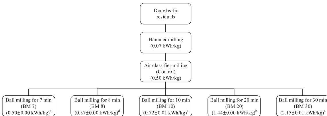
Fig. 1. Process flow diagram and energy consumption of each milling process set used. Different alphabet superscripts indicates that means of energy input for ball milling were significantly different ( $p < .05$ ).
