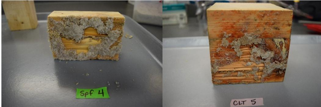
Figure 3. Termite excavations on the exposed (bottom) face of spruce/pine/fir and CLT test blocks. Termites and mud tubes intact on test blocks.
