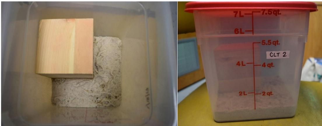
Figure 1. Test containers for subterranean termite testing. Termites introduced into corner diagonally opposite of the test block location.
