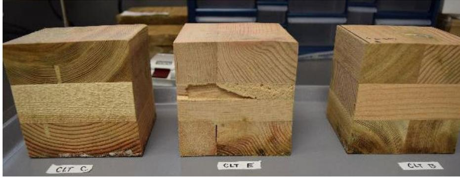
**Figure 2. Water staining on exposed (bottom) face of control (no termite) CLT blocks after 8 weeks. Average water uptake of control blocks was 39.5 g.**
