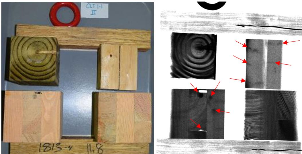
Figure 4. X-ray scan analysis. Red arrows on right indicate suspected termite damage areas. Top left = copper azole treated pine; Top right = spruce/pine/fir; Bottom left = CLT exposed to termites; Bottom right = CLT control.
