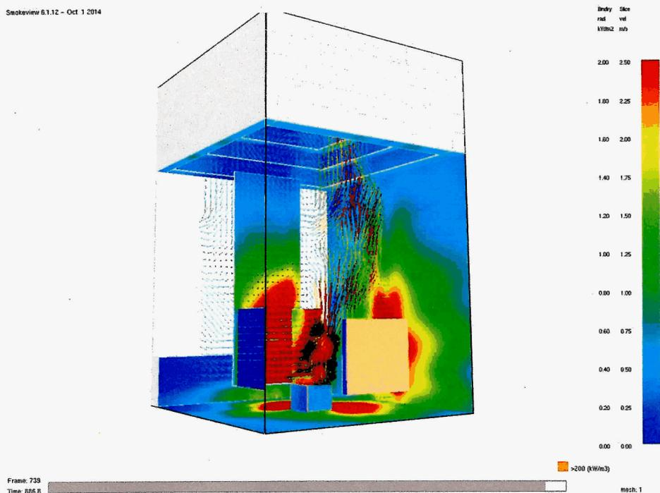
Figure 2 Propane pool fire under HRR hood with opened North wall with FDS rendition of flows and radiant heat fluxes from 30% radiant fraction of HRR measured with advanced O<sub>2</sub> consumption method corrected for CO<sub>2</sub>, CO, H<sub>2</sub>O and soot measurements
