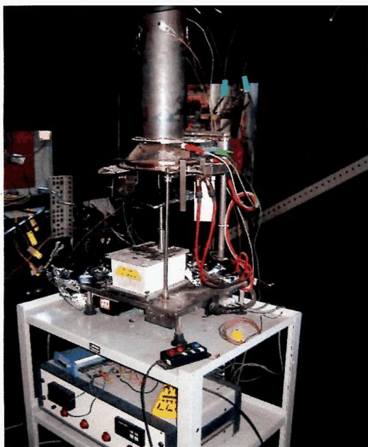
Figure 1 Modified MLC under FPL's HRR hood surrounded by radiant absorbing walls
