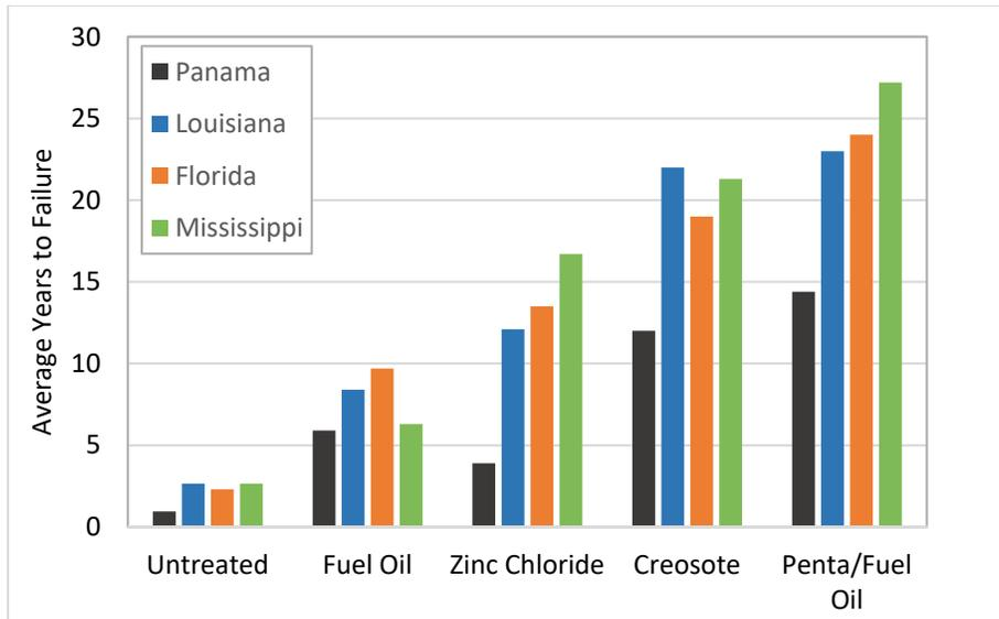
**Figure 1. Examples of the longevity of matched stakes exposed in Panama or sites in the southeastern US. The creosote and pentachlorophenol treated stakes depicted here do not meet AWPA standards and this data does not reflect the expected longevity of commodities currently treated with these preservatives.**
