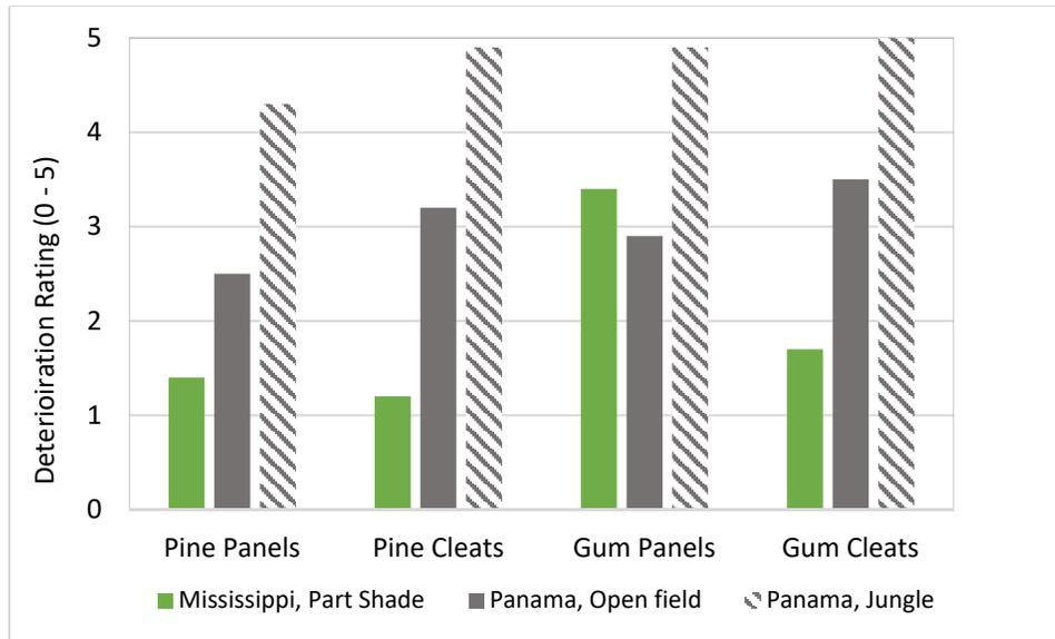
**Figure 3. Mean deterioration ratings for untreated wooden boxes exposed in Mississippi or Panama. Boxes were rated on a scale from 0 (no attack) to 5 (destroyed). The exposure period was 47 months in Mississippi and 36 months in Panama.**
