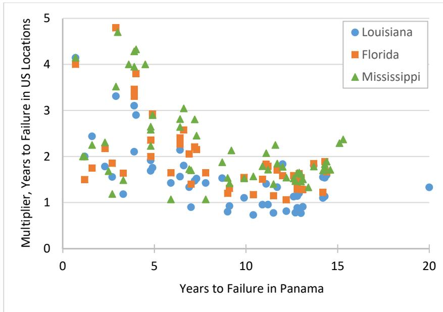
**Figure 2. Longevity of stakes exposed in sites within the southeastern US relative to those exposed in Panama. Y-axis represents the ratio, Years to failure in US sites/Years to failure in Panama. Note that the general trend is that the ratio of early failures is many times greater in US sites, but for later failures the ratios are much lower.**
