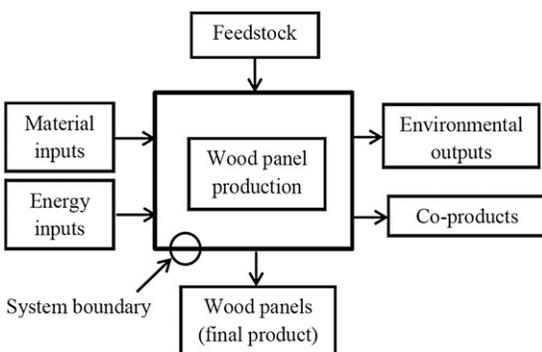
Figure 3. Process flow diagram for wood panel production.
