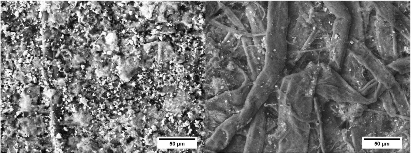
Figure 2.—Scanning electron microscope images of the paper after (left) and before (right) the application of the radiative reflective coating.
