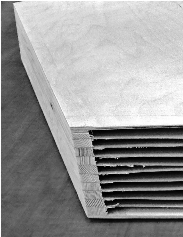
Figure 3.—Laboratory-scale Mirrorpanel that was later sectioned to show the construction technique.
