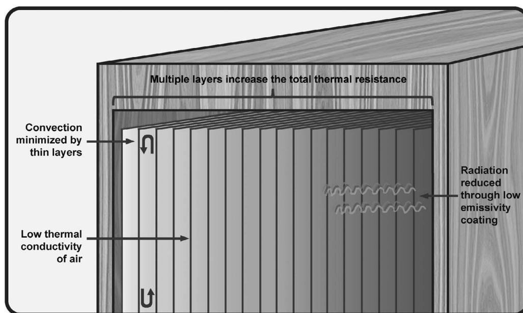
Figure 1.—Schematic drawing of how the Mirrorpanel reduces the three methods of heat transfer and provides insulation.
