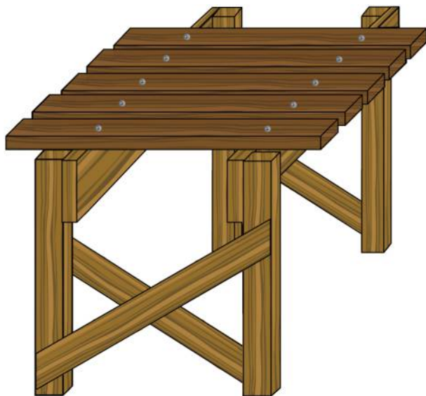
1 Sketch of test set-up for exposure of decking specimens
