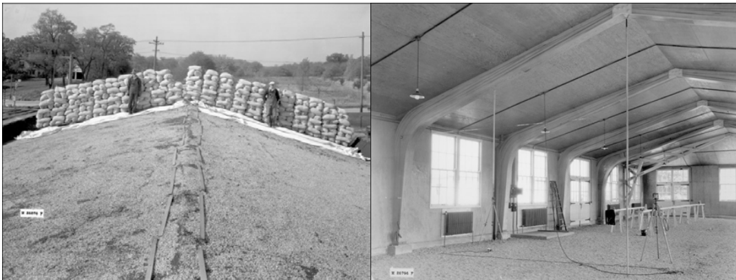
Figure 3 — Loading of arch building and measurement techniques for live loading of building.
