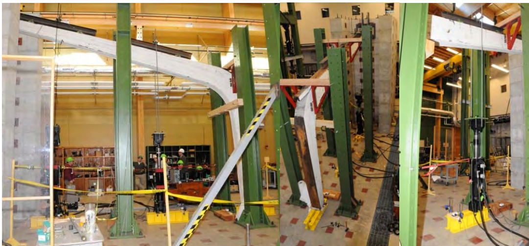
Figure 6 —Testing setup of one half of single arch with a four-point loading configuration.
