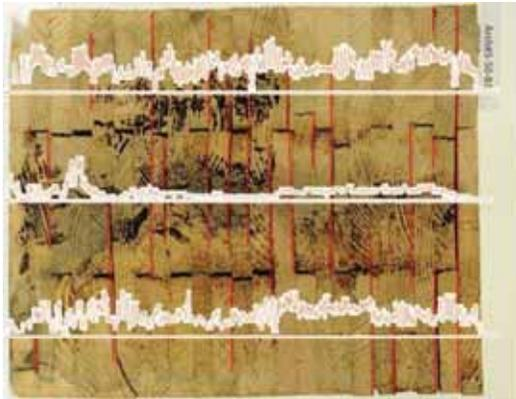
**Figure 6**— Image of the glulam cross-section at location 1 superimposed with the resistance profile of three drilling paths (Red lines indicate delamination by visual inspection).
