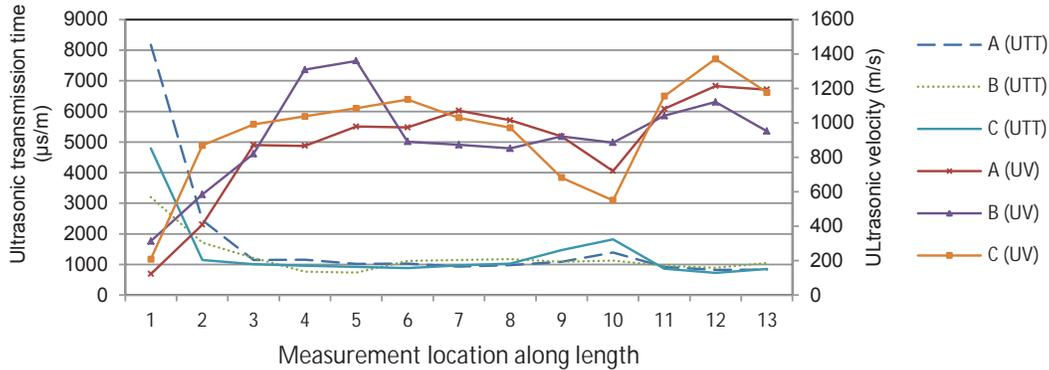
**Figure 4**—Ultrasonic transmission time and ultrasonic velocity measured across laminations of the glulam arch section (Notes: UTT – ultrasonic transmission time, UV – ultrasonic velocity).
