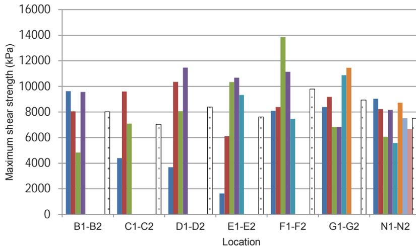
**Figure 10**—Maximum shear strength of small samples obtained from the glulam arch (Note: shaded columns indicate mean values).
