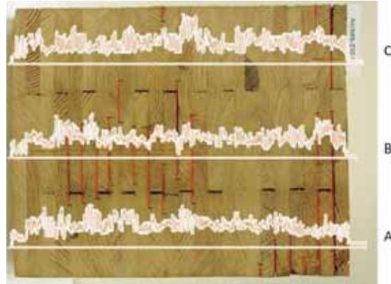
**Figure 7**— Image of the glulam cross-section at location 2 superimposed with the resistance profile of three drilling paths (Red lines indicate delamination by visual inspection).
