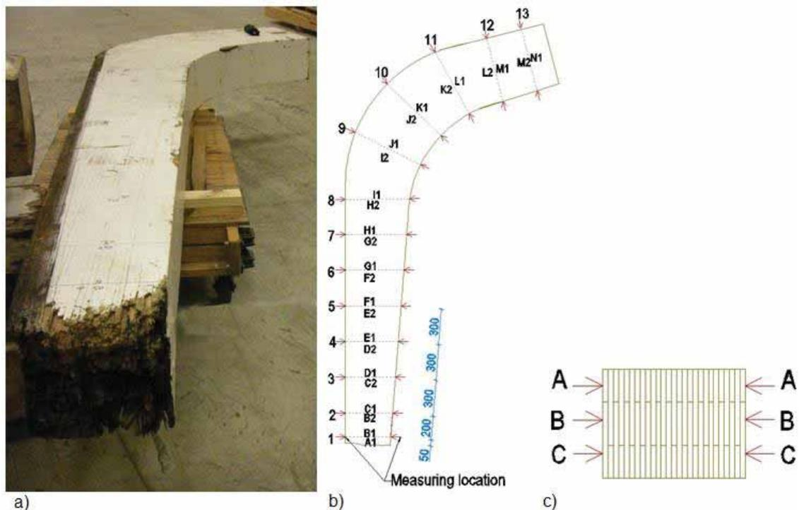
**Figure 2**—a) Glulam arch under testing; b) Plan view showing measurement locations; c) Cross-section view showing measurement locations (A, B, and C were 45, 135 and 225 mm from the edge of the cross-section respectively).
