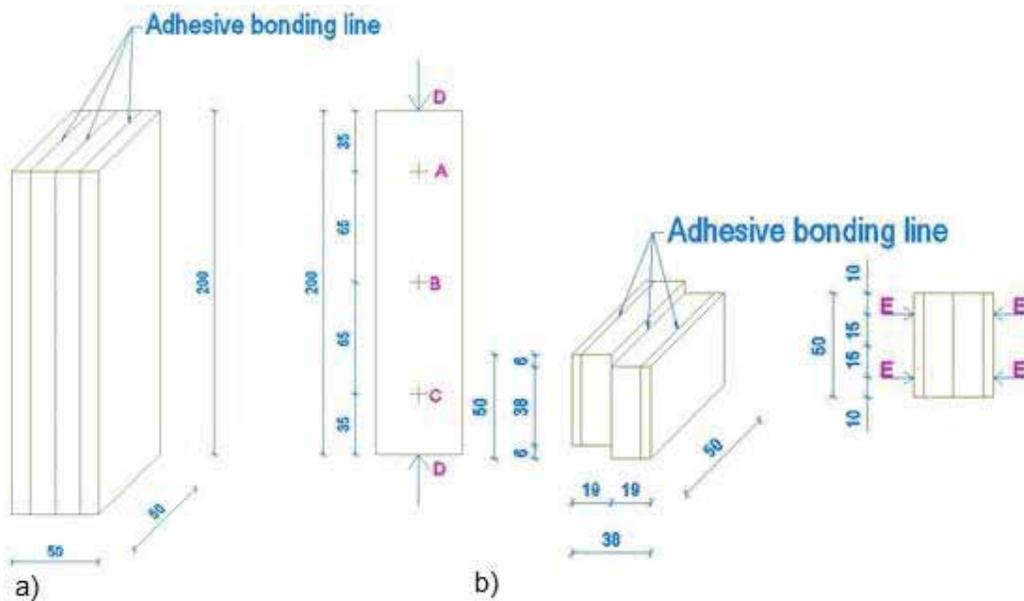
**Figure 3**—Small samples cut from the glulam blocks for mechanical testing. a) Compression test sample with ultrasonic measurements at point A, B, C and D; b) Shear test sample with ultrasonic measurement at point E.
