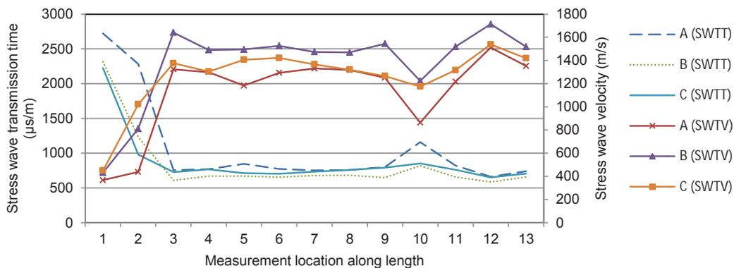
**Figure 5**—Stress wave transmission time and stress wave velocity measured across laminations of the glulam arch section (Notes: SWTT – stress wave transmission time, SWTV – stress wave transmission velocity).
