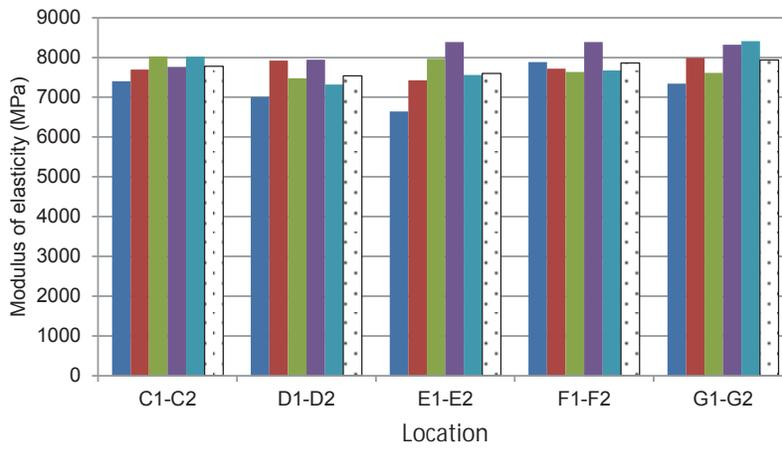
**Figure 9**—Modulus of elasticity (in compression) of small samples obtained from the glulam arch (Note: shaded columns represent mean values).
