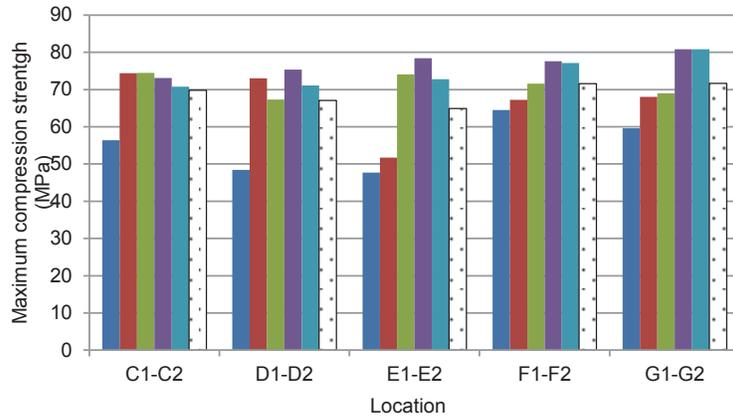
**Figure 8**—Maximum compression strength (parallel to grain) of small samples obtained from the glulam arch (Note: Shaded columns represent mean values).
