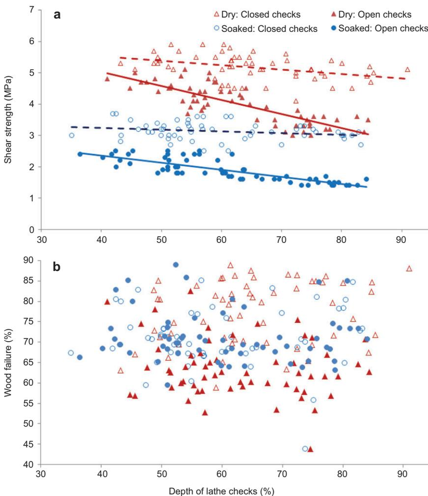
**Figure 2** (a) Shear strength values of tested plywood under dry and wet conditions pulling checks open or closed. (b) Effect of depth of lathe checks on percentage of wood failure evaluated by automated image analysis for checks pulled open and closed under wet and dry conditions.
