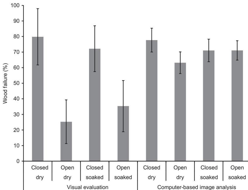
**Figure 3** Percentage of wood failure evaluated by different methods. Error bars represent one standard deviation.
