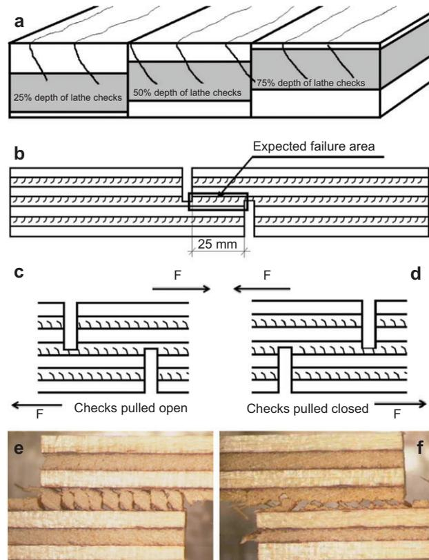
**Figure 1** (a) Schematic representation of the three veneer groups to control check depth (the shaded area is the final veneer after sanding). (b) Schematic visualization of plywood shear test configuration and bondline under test. (c) Middle ply with lathe checks pulled open. (d) Middle ply with lathe checks pulled closed. (e) Plywood failure in open fashion. (f) Plywood failure closed fashion. (The loose side of the tested veneer is at the bottom of c–f.)
