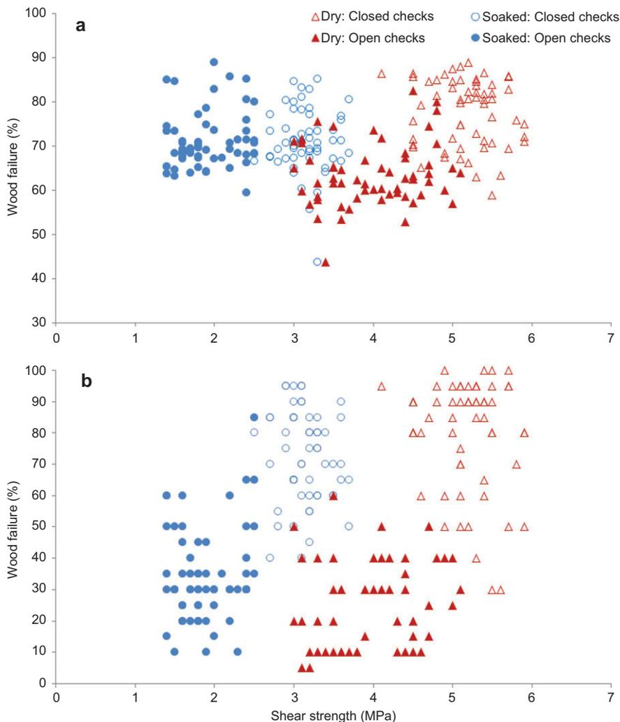
**Figure 4** (a) Relationship between shear strength and wood failure of plywood evaluated by an automated image analysis for checks pulled open and closed under wet and dry conditions. (b) Relationship between shear strength and wood failure of plywood evaluated visually for checks pulled open and closed under wet and dry conditions.
