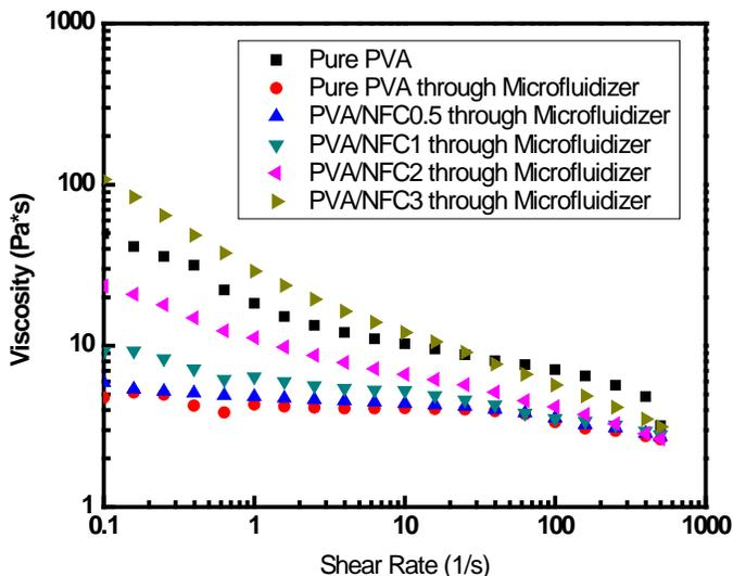
Figure 2. The viscosity curves of pure PVA and PVA/NFC solutions with respect to shear rate.
