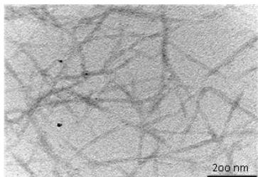
Figure 1. TEM image of TEMPO-oxidized cellulose with a concentration of 0.5 wt %.
