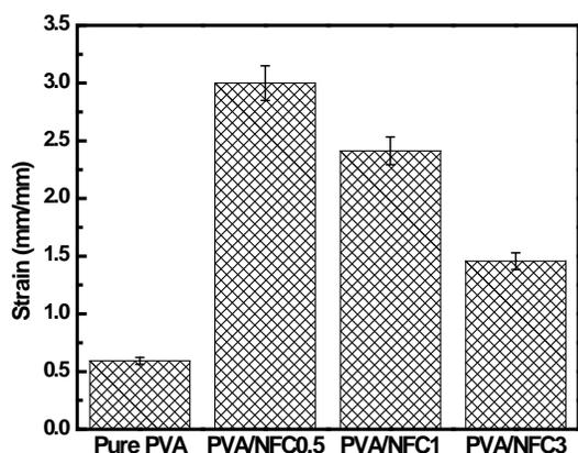
Figure 5. Strain-at-break of pure PVA and PVA/NFC filaments with different NFC contents.
