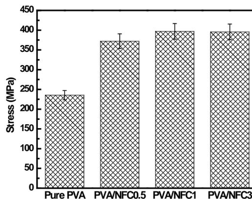
Figure 4. Ultimate tensile strength of pure PVA and PVA/NFC filaments with different NFC contents.
