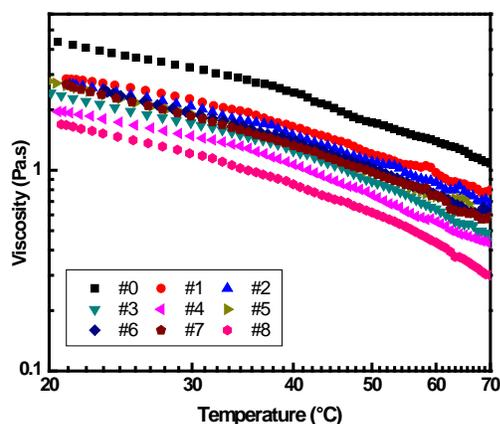
Figure 8. PVA solution viscosities corresponding to various processing conditions with respect to temperature.
