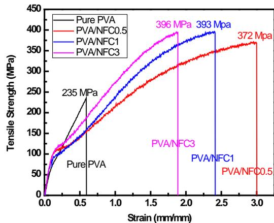
Figure 3. The mechanical properties of pure PVA and PVA/NFC filaments. The numbers 0.5, 1, and 3 refer to the NFC content in the PVA matrix.
