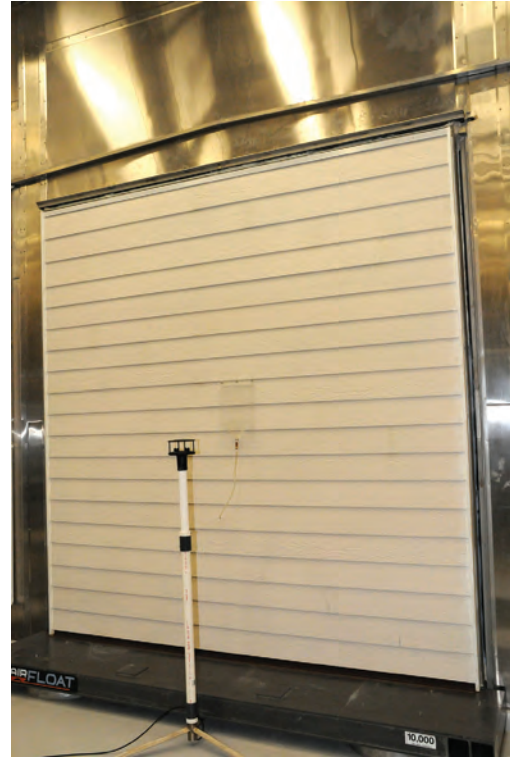
Figure 4 Wall installed between indoor and outdoor chambers, with wind and rain gauges.
