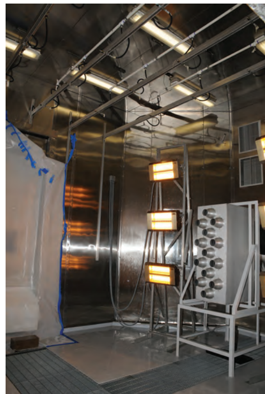
Figure 5 CARWASH wind array, also showing IR heaters and rain spray nozzles overhead.
