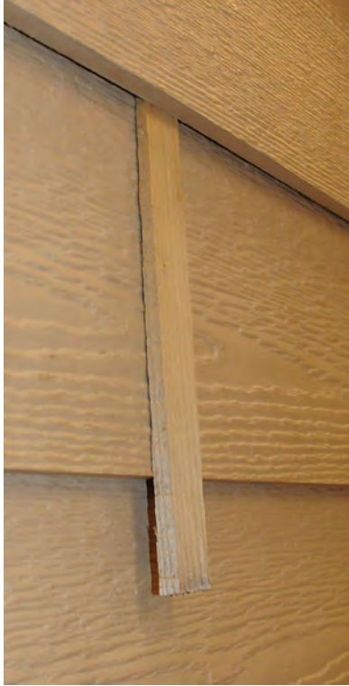
Figure 9 Wedge to create defect in lap siding.
