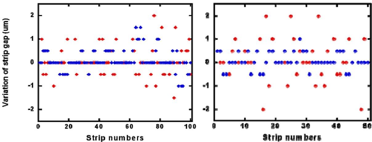
Figure 3: Thermal expansion measured by variation of SiNM strip gaps before (left) and after (right) heating; the red markers represent vertical alignment and the blue represent horizontal
