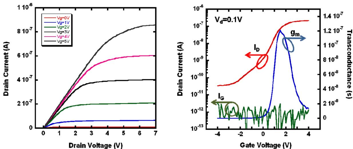
Figure 6: Electrical characteristics of the device.  $V_g$ : Gate voltage;  $I_d$ : drain current;  $g_m$ : transconductance;  $V_d$ : drain voltage.
