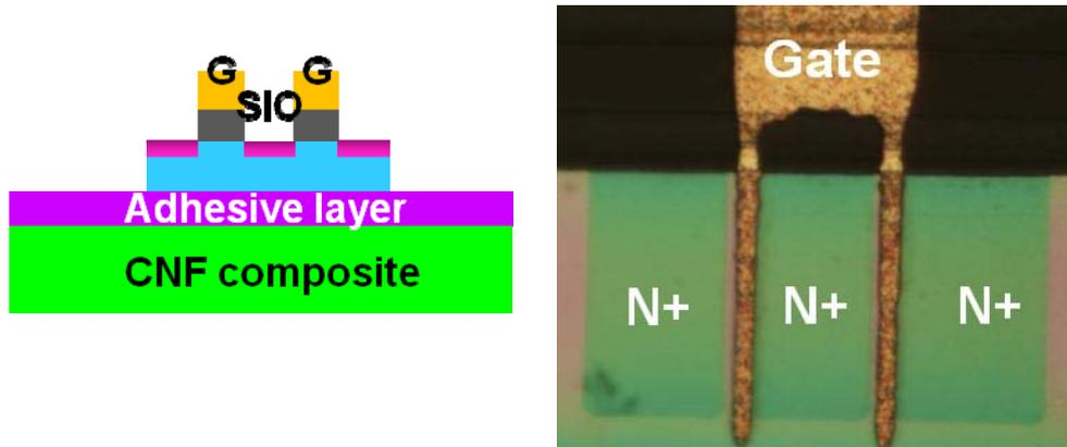
Figure 4: Schematic and micrograph of the gate stack. N+: doped area; G: gate.
