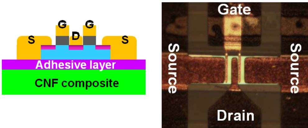
Figure 5: Schematic and micrograph of the final TFT device. S: source; G: gate; D: drain.
