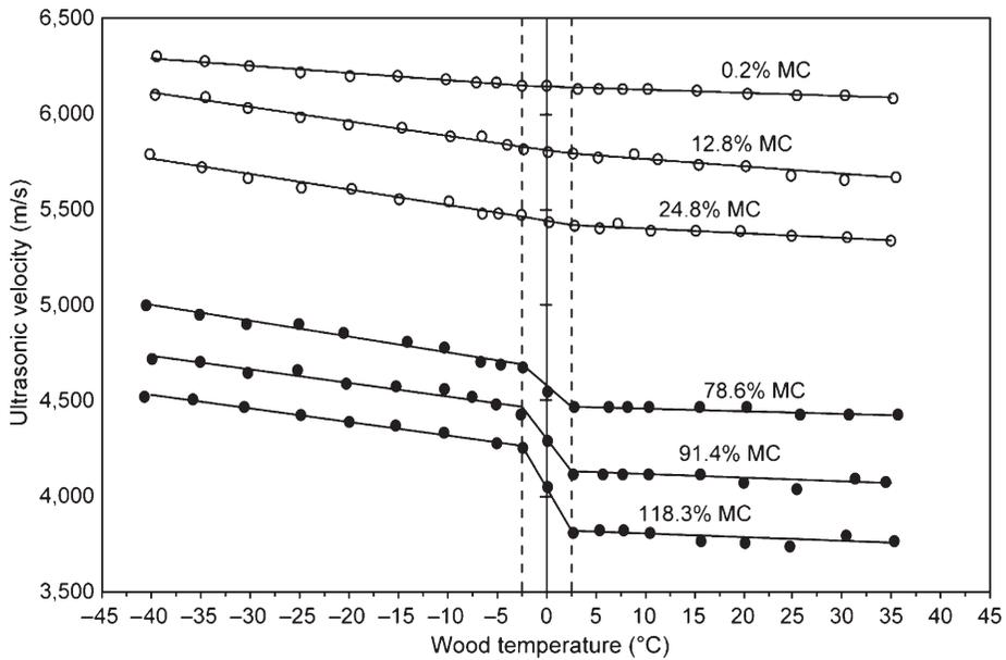
Figure 4. Plot of ultrasonic velocity of red pine as a function of wood temperature at different moisture content (MC) levels.
