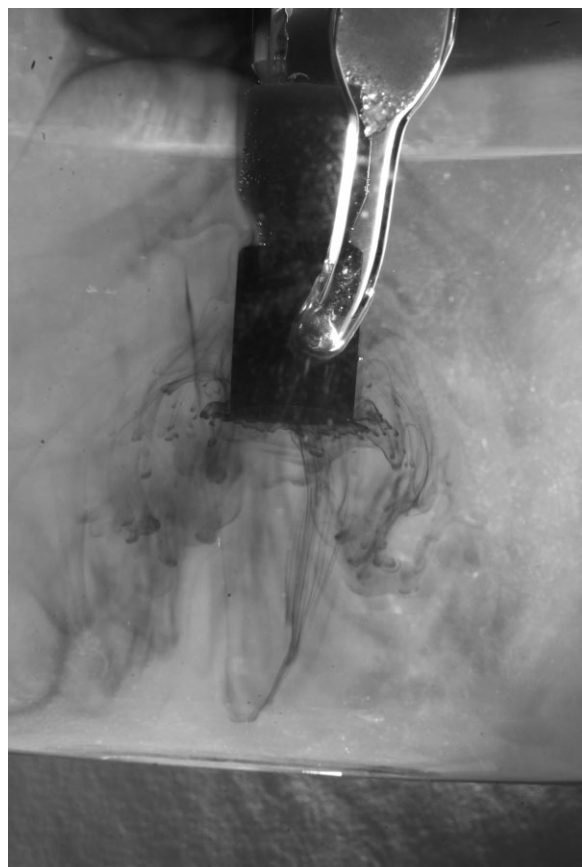
Figure 1. Blue-black precipitate forming on the surface of the steel plug exposed to synthetic oak extract
