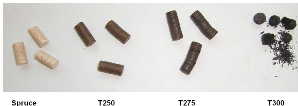
Fig. 5 – Pellets made from spruce and torrefied spruce. From left to right: Spruce and torrefied spruce at 250, 275 and 300 °C.
