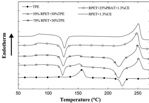
FIG. 2. Melting curves of the PET blends. Data obtained from the first heating cycle.
