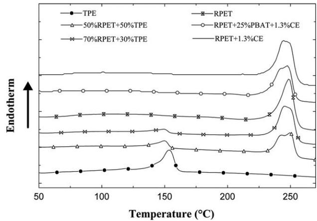
FIG. 3. Melting curves of the RPET blends. Data obtained from the second heating cycle.
