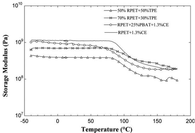
FIG. 9. Storage moduli of the RPET blends after heat treatment.
