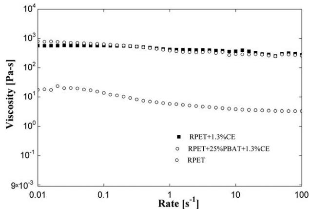
FIG. 11. Flow curves for RPET-CE and PET-PBAT-CE blends ( $T = 260^\circ\text{C}$ ).
