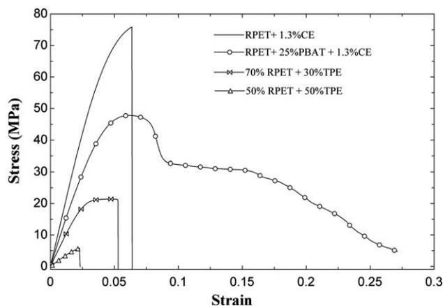
FIG. 6. Tensile stress versus strain curves for the RPET blends after heat treatment.
