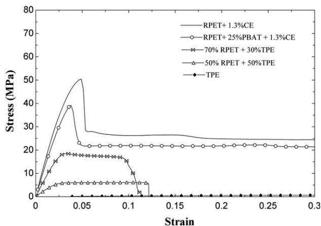
FIG. 5. Tensile stress versus strain curves for the TPE and RPET blends.
