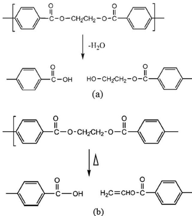
FIG. 1. (a) Hydrolytic and (b) thermal degradation reactions of PET.
