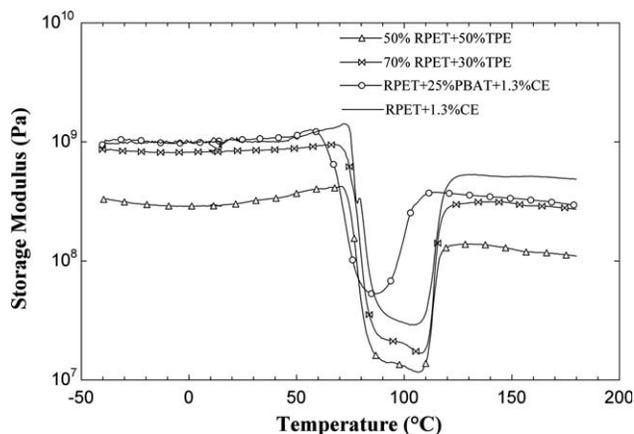
FIG. 7. Storage moduli of the RPET blends for specimens cut directly from injection molded tensile test bars.
