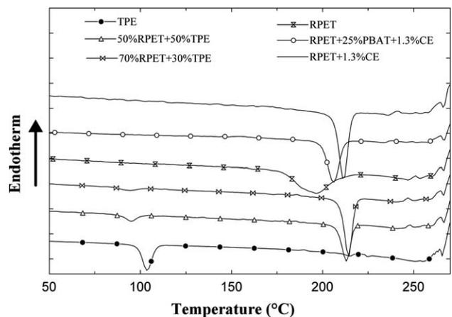
FIG. 4. Melting curves of the RPET blends. Data obtained from the cooling cycle.
