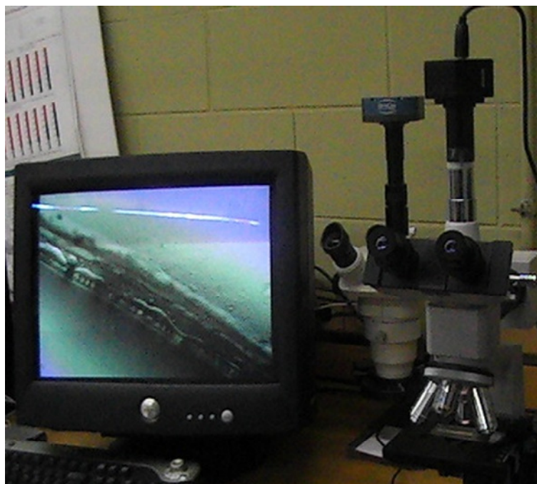
Figure 3: Studying the swelling of CNF films under an optical microscope
