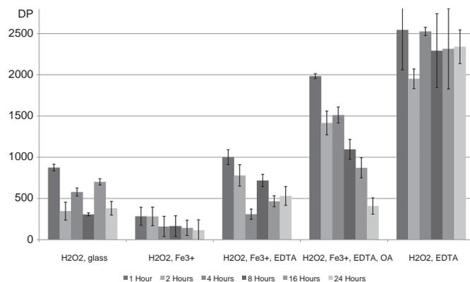
**Fig. 2.** Treatment of cotton with H<sub>2</sub>O<sub>2</sub> (80 mM) and combinations of glass, Fe(SO<sub>4</sub>)<sub>3</sub>, EDTA, and OA over a period of 1–24 h of exposure. The degree of polymerization of untreated cotton cellulose control samples at time zero were 2181 ± 117 DP ( $n = 3$ ). The average DP of dH<sub>2</sub>O-treated control measured at time 1–24 h was 1970 ± 71 DP ( $n = 18$ ).
