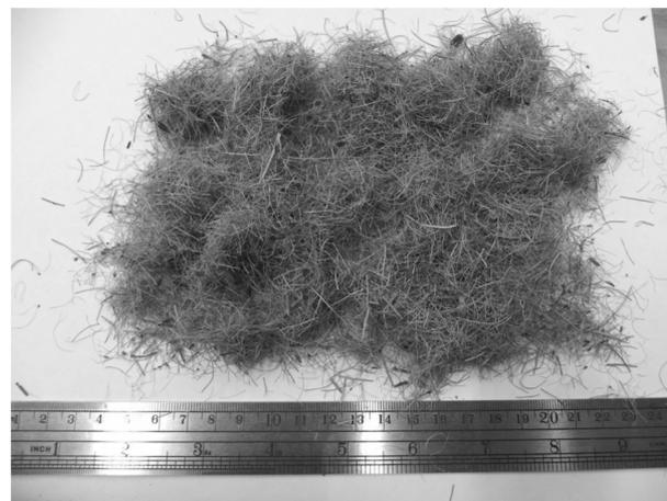
**Figure 1.** Hammer-milled coir (coconut) fibers used in the manufacture of the reinforced polypropylene composite panel.
