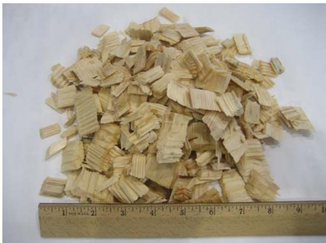
**Fig. 1** Lodgepole pine wood chips directly used in SPORL chemical pretreatment process
