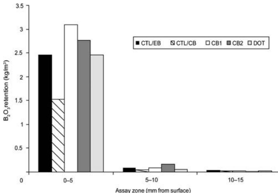
Figure 4.—Boron retention, as  $B_2O_3$ , for each assay zone. Values for the three target moisture contents were averaged. CTL/EB = chlorothalonil/experimental glycol-borate, CTL/CB = chlorothalonil/commercial glycol-borate, CB = commercial glycol-borate, DOT = disodium octaborate tetrahydrate.
