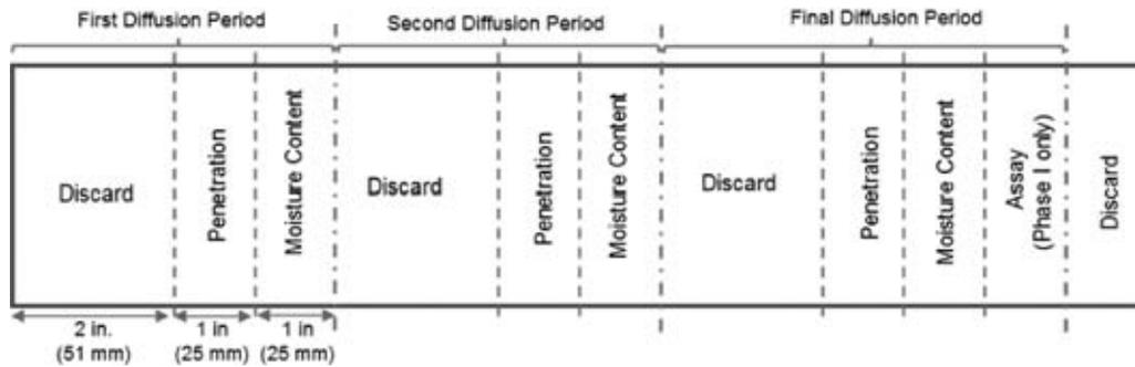
Figure 2.—Pattern used for cutting penetration, moisture content, and assay samples from specimens (top view). Diffusion periods were 2, 4, and 8 weeks for Phase I and 6, 13, and 26 weeks for Phase II.
