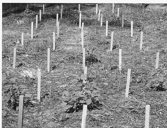
Fig. 4 In-ground field test of WPC specimens [1.9 cm × 45.7 cm (0.75 in. × 18 in.)] in Saucier, Mississippi.
