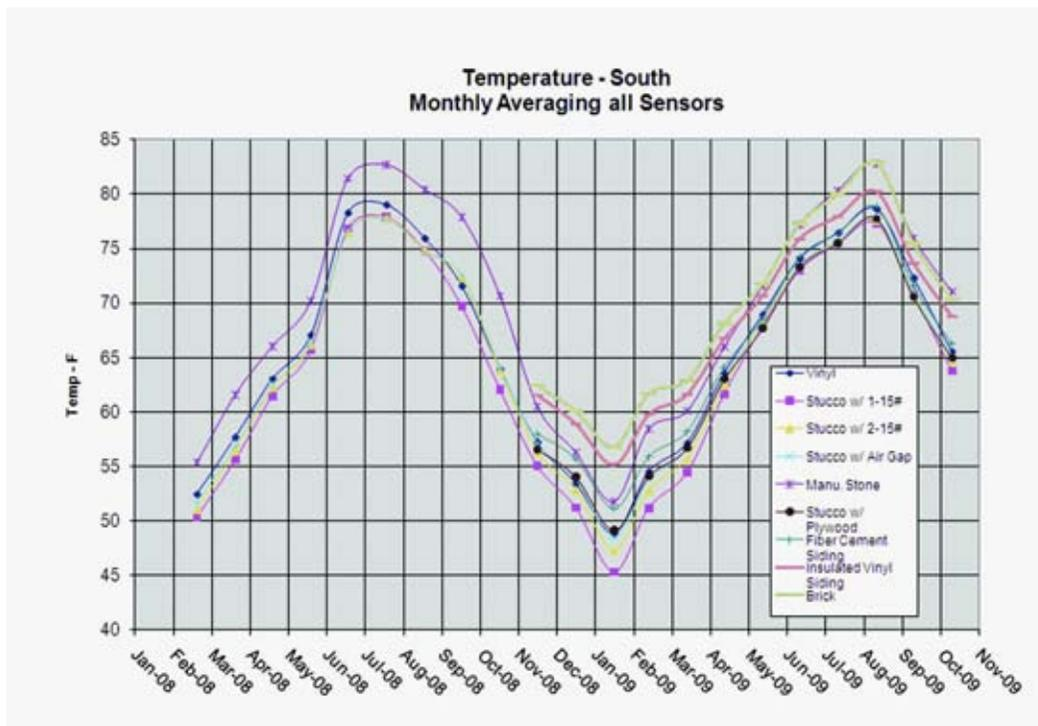
**Figure 6** Wall cavity temperature: south.
