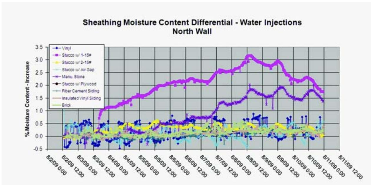
**Figure 9** Sheathing moisture content increase with water injections: north. Note: stucco wall with plywood readings were determined to be unreliable, and thus were not reported on this graph.
