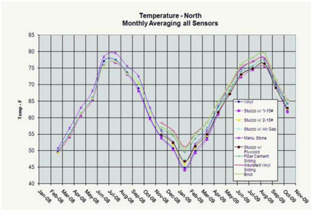
Figure 7 Wall cavity temperature: north.
