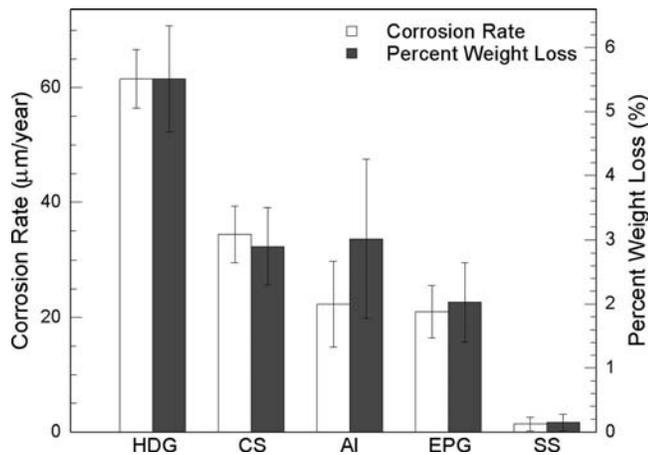
**Fig. 2.** Results of the corrosion tests conducted in a 27°C, 100% relative humidity environment in ACQ treated wood for a hot-dip galvanized nail (HDG), carbon steel nail (CS), electroplated galvanized screw (EPG), aluminum nail (AI) and a stainless steel nail (SS). The values represent the average of nine replicates, which were exposed from times between 36 and 48 weeks. The error bars represent the uncertainty in the mean.
