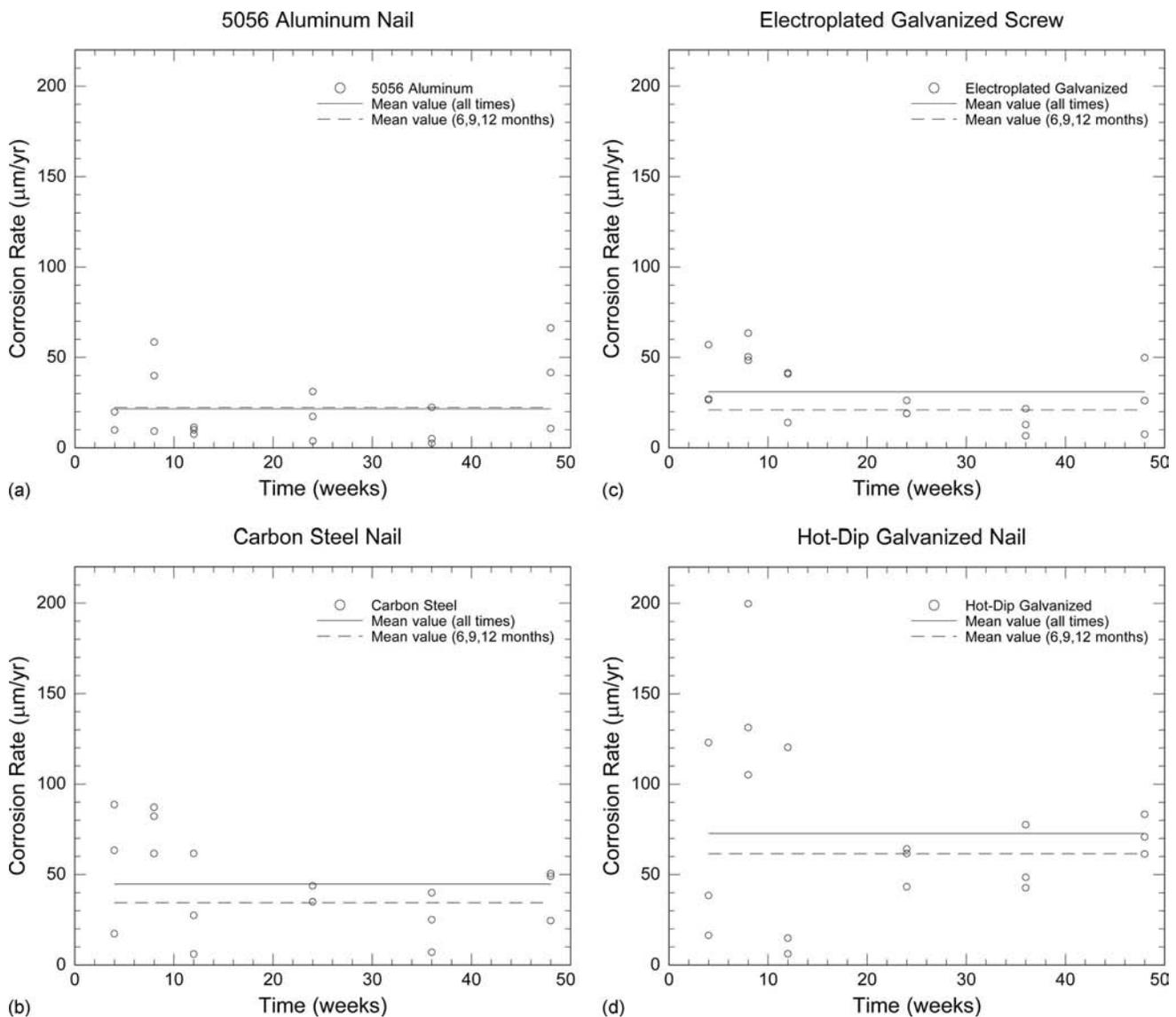
**Fig. 1.** Corrosion rate (in  $\mu\text{m}/\text{year}$ ) for fasteners exposed to ACQ treated wood for various times: (a) 5056 aluminum nail; (b) carbon steel nail; (c) electroplated galvanized screw; and (d) hot-dip galvanized nail. Solid line represents the mean value over all times, the dashed line represents the mean corrosion rate collected from times after 6 months (48 weeks).
