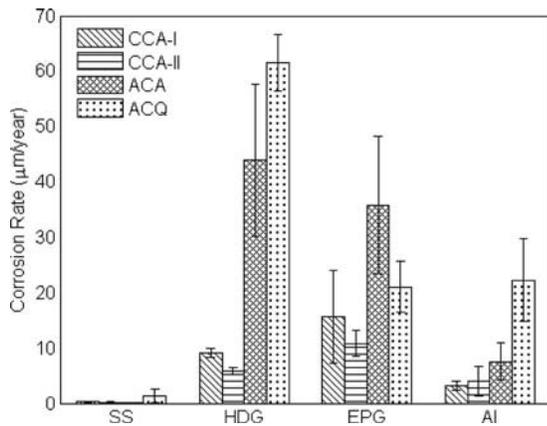
**Fig. 3.** Corrosion rates of metals exposed to treated wood. The error bars represent the uncertainty in the mean.
