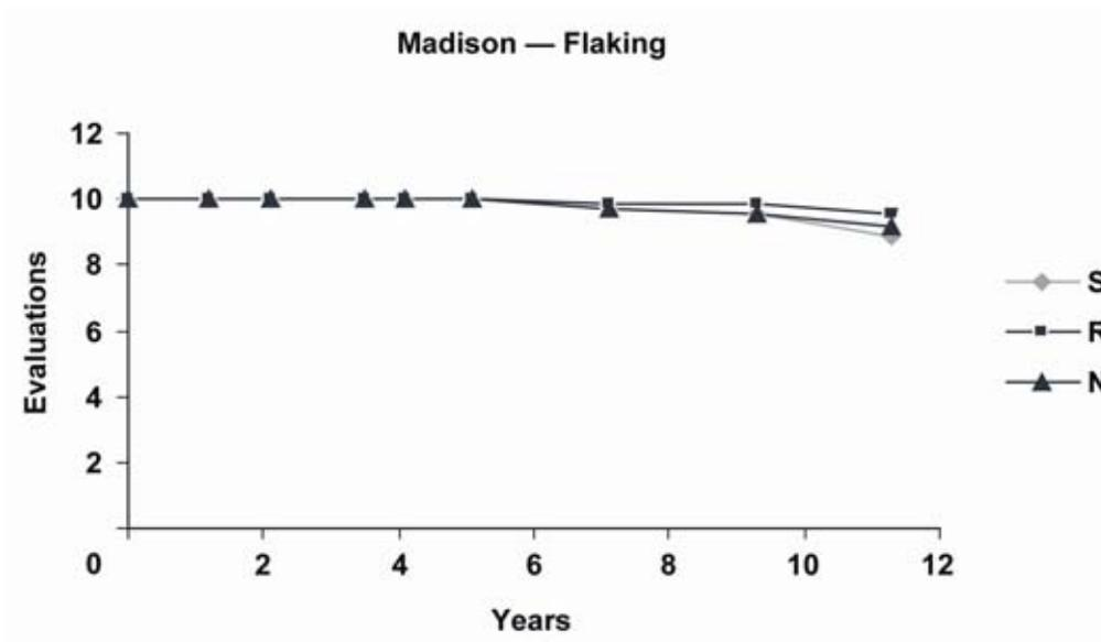
Figure 17. Paint flaking evaluations: average of all paint systems over 11 years outdoor exposure near Madison, Wisconsin. Primer surface treatment: S, sanding and washing; R, repriming; N, nothing (finishing “as is”).
