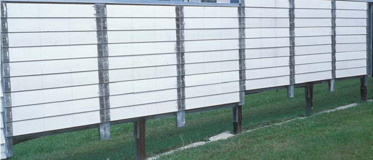
Figure 2. Boards mounted on test fence near Madison, Wisconsin, after several years of outdoor exposure.
