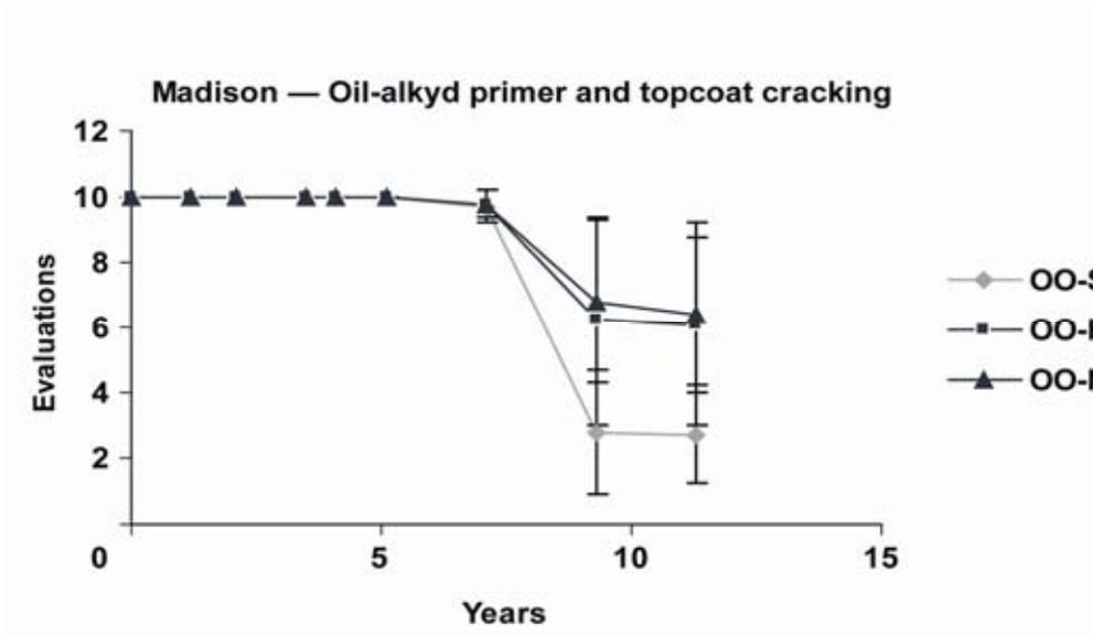
Figure 21. Paint cracking evaluations of oil-alkyd primer and topcoat (OO) over 11 years exposure near Madison, Wisconsin. Primer surface treatment: S, sanding and washing; R, repriming; N, nothing (finishing "as is").
