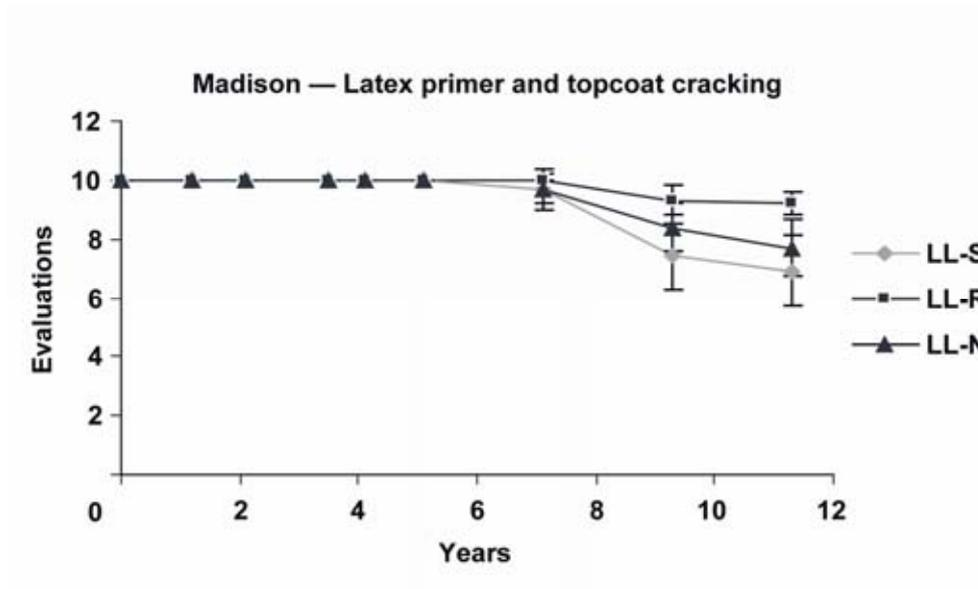
Figure 19. Paint cracking evaluations of latex primer and topcoat (LL) over 11 years exposure near Madison, Wisconsin. Primer surface treatment: S, sanding and washing; R, repriming; N, nothing (finishing “as is”).
