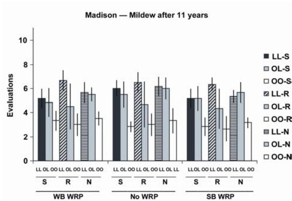
Figure 5. Mildew evaluations of painted western redcedar following 11 years outdoor exposure near Madison, Wisconsin (average of six replicates and error-bar is the first standard deviation). Paint systems: LL, latex primer and topcoat; OL, oil-alkyd primer/latex topcoat; OO, oil-alkyd primer and topcoat. Primer surface treatment: S, sanding and washing; R, repriming; N, nothing (finishing “as is”).
