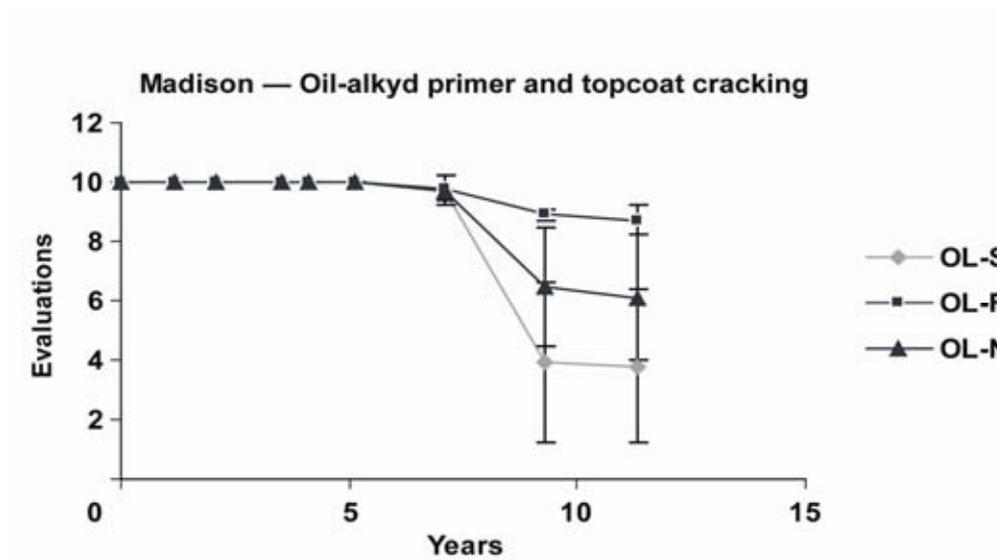
Figure 20. Paint cracking evaluations of oil-alkyd primer/latex topcoat (OL) over 11 years exposure near Madison, Wisconsin. Primer surface treatment: S, sanding and washing; R, repriming; N, nothing (finishing “as is”).
