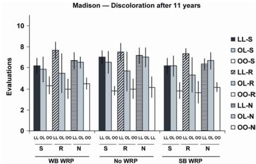
Figure 4. Discoloration evaluations of painted western redcedar following 11 years outdoor exposure near Madison, Wisconsin. Shown is the average of six replicates. The error bar is the first standard deviation. Paint systems: LL, latex primer and topcoat; OL, oil-alkyd primer/latex topcoat; OO, oil-alkyd primer and topcoat. Primer surface treatment: S, sanding and washing; R, repriming; N, nothing (finishing “as is”).
