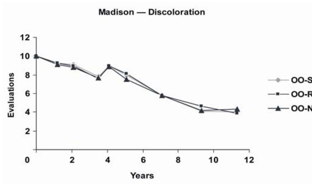
Figure 12. Paint discoloration evaluations of oil-alkyd primer and topcoat (OO) over 11 years outdoor exposure near Madison, Wisconsin. Primer surface treatment: S, sanding and washing; R, repriming; N, nothing (finishing “as is”). Average of data for water-based preservative (WPR) and no WPR treatment .
