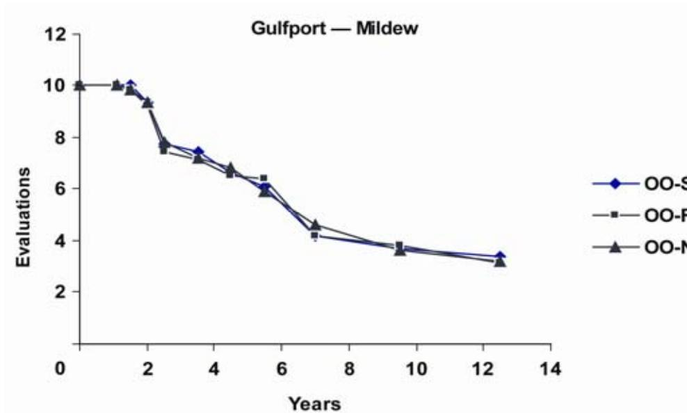
Figure 14. Mildew evaluations of oil-alkyd primer and topcoat (OO) over 12 years outdoor exposure near Gulfport, Mississippi. Primer surface treatment: S, sanding and washing; R, repriming; N, nothing (finishing “as is”). Average of data for water-repellent preservative (WRP) and no WRP treatment.
