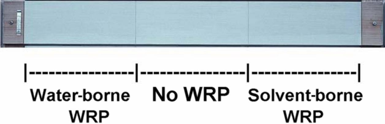
Figure 1. Sample of single painted board showing the water-repellent preservative (WRP) treatment.
