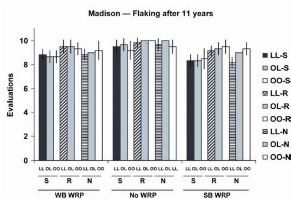
Figure 6. Flaking evaluations of painted western redcedar following 11 years outdoor exposure near Madison, Wisconsin (average of six replicates and error-bar is the first standard deviation). Paint systems: LL, latex primer and topcoat; OL, oil-alkyd primer/latex topcoat; OO, oil-alkyd primer and topcoat. Primer surface treatment: S, sanding and washing; R, repriming; N, nothing (finishing “as is”).
