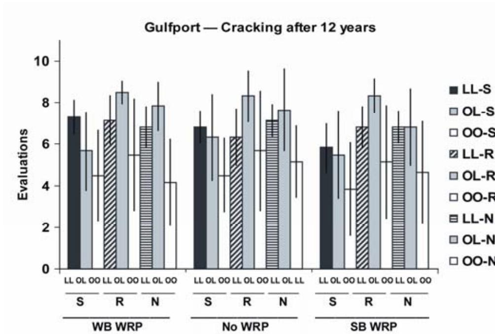
Figure 11. Cracking evaluations of painted western redcedar following 12 years outdoor exposure near Gulfport, Mississippi (average of six replicates and error-bar is the first standard deviation). Paint systems: LL, latex primer and topcoat; OL, oil-alkyd primer/latex topcoat; OO, oil-alkyd primer and topcoat. Primer surface treatment: S, sanding and washing; R, repriming; N, nothing (finishing “as is”).
