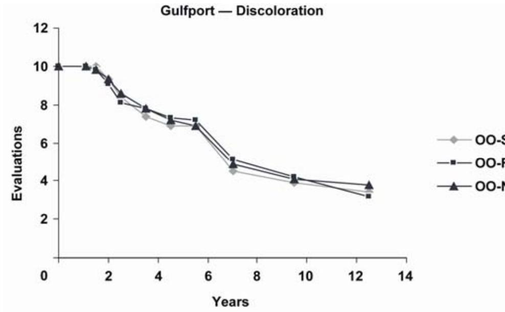
Figure 13. Paint discoloration evaluations of oil-alkyd primer and topcoat (OO) over 12 years outdoor exposure near Gulfport, Mississippi. Primer surface treatment: S, sanding and washing; R, repriming; N, nothing (finishing “as is”). Average of data for water-repellent preservative (WRP) and no WRP treatment.
