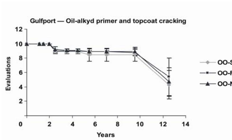
Figure 22. Paint cracking evaluations of oil-alkyd primer and topcoat (OO) over 12 years exposure near Gulfport, Mississippi. Primer surface treatment: S, sanding and washing; R, repriming; N, nothing (finishing "as is").
