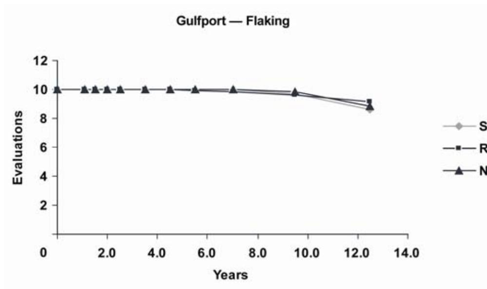
Figure 18. Paint flaking evaluations: average of all paint systems over 12 years outdoor exposure near Gulfport, Mississippi. Primer surface treatment: S, sanding and washing; R, repriming; N, nothing (finishing “as is”).
