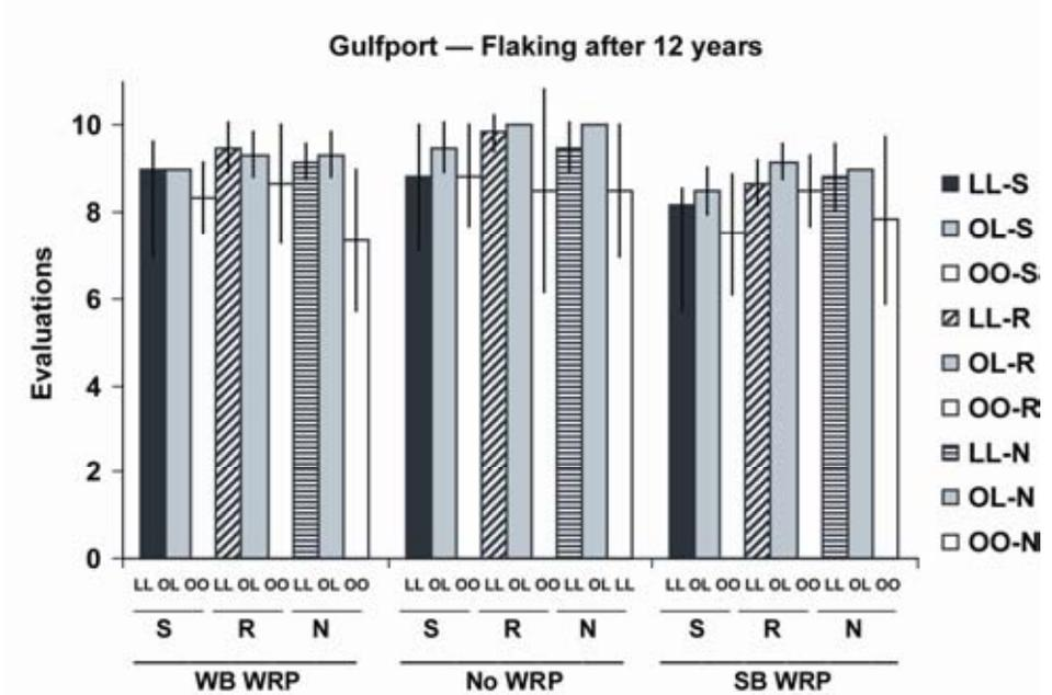
Figure 10. Flaking evaluations of painted western redcedar following 12 years outdoor exposure near Gulfport Mississippi (average of six replicates and error-bar is the first standard deviation). Paint systems: LL, latex primer and topcoat; OL, oil-alkyd primer/latex topcoat; OO, oil-alkyd primer and topcoat. Primer surface treatment: S, sanding and washing; R, repriming; N, nothing (finishing “as is”).
