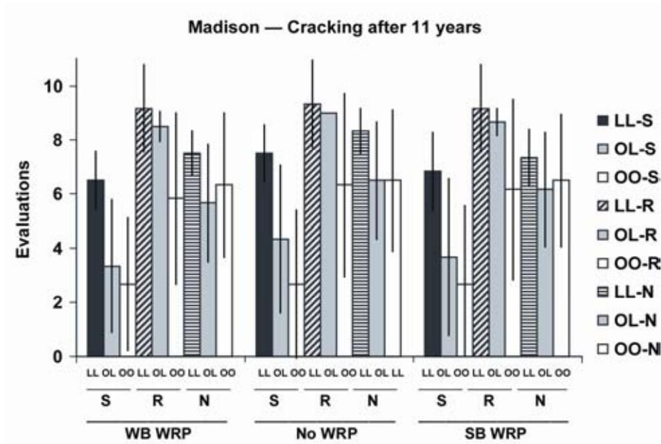
Figure 7. Cracking evaluations of painted western redcedar following 11 years outdoor exposure near Madison Wisconsin (average of six replicates and error-bar is the first standard deviation). Paint systems: LL, latex primer and topcoat; OL, oil-alkyd primer/latex topcoat; OO, oil-alkyd primer and topcoat. Primer surface treatment: S, sanding and washing; R, repriming; N, nothing (finishing “as is”).
