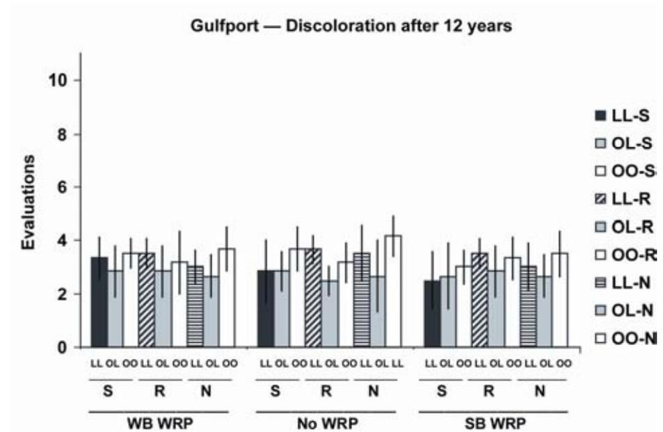
Figure 8. Discoloration evaluations of painted western redcedar following 12 years outdoor exposure near Gulfport, Mississippi (average of six replicates and error-bar is the first standard deviation). Paint systems: LL, latex primer and topcoat; OL, oil-alkyd primer/latex topcoat; OO, oil-alkyd primer and topcoat. Primer surface treatment: S, sanding and washing; R, repriming; N, nothing (finishing “as is”).
