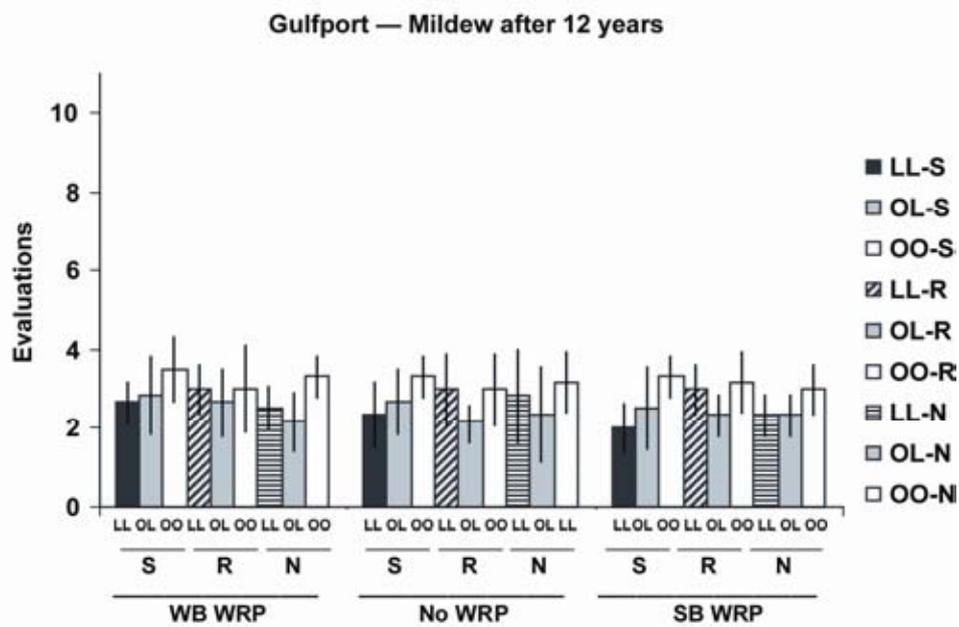
Figure 9. Mildew evaluations of painted western redcedar following 12 years outdoor exposure near Gulfport, Mississippi (average of six replicates and error-bar is the first standard deviation). Paint systems: LL, latex primer and topcoat; OL, oil-alkyd primer/latex topcoat; OO, oil-alkyd primer and topcoat. Primer surface treatment: S, sanding and washing; R, repriming; N, nothing (finishing “as is”).
