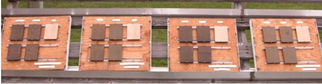
**Figure 3:** Outdoor weathering of sol-gel-treated and non-treated (control) wood specimens.
