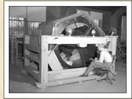
Testing box materials and construction for durability helped revolutionize the shipping industry during and after World War I.
