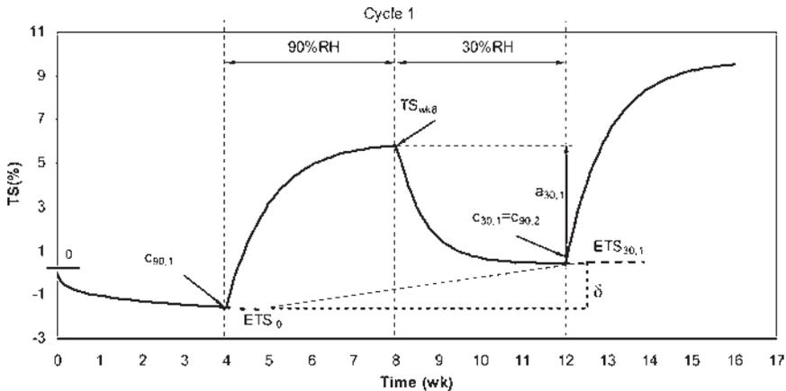
Figure 5. Exponential model curve of thickness swelling (TS) for unsealed oriented strandboard: Cycle 1. ETS: equilibrium TS;  $\delta$  = difference in ETS values between end and beginning of one cycle.  $a_{90}$ : coefficient a from Eq 6a;  $a_{30}$ : coefficient a from Eq 6b.
