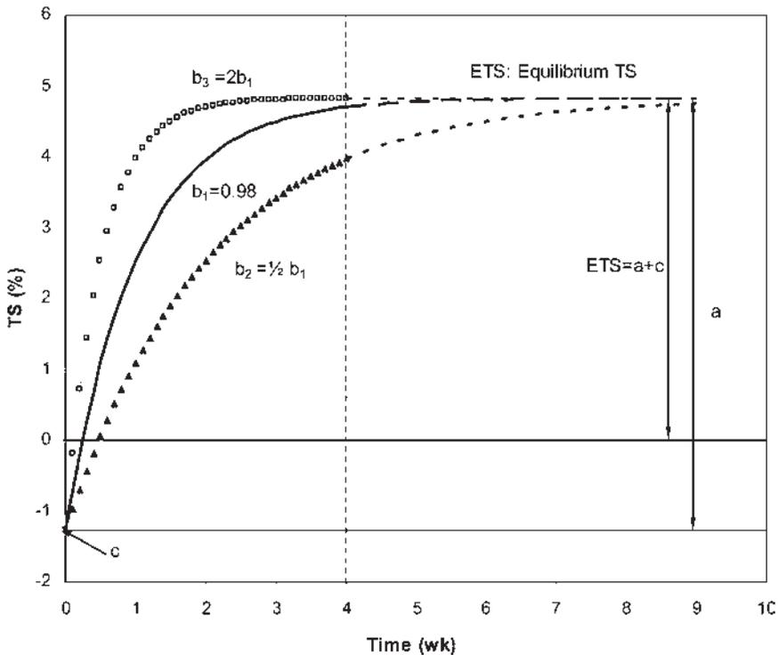
Figure 4. Thickness swelling (TS) curve for illustrating effect of coefficient  $b$  based on Eq 6a:  $TS = c + a[1 - \exp(-bt)]$ .
