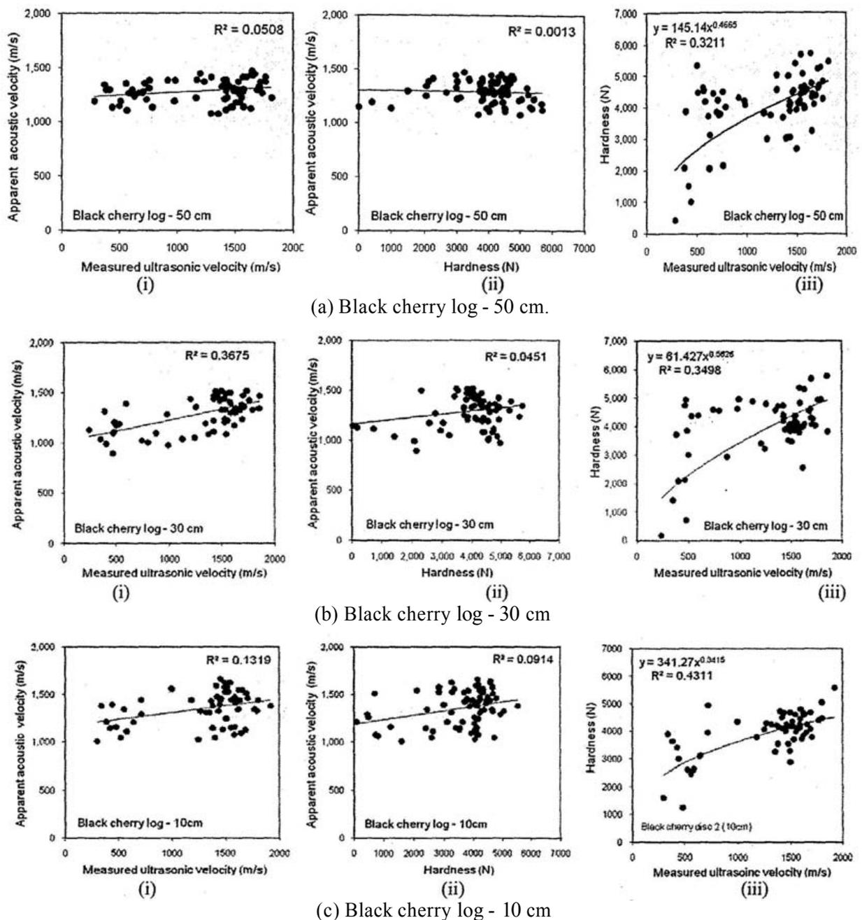
**Figure 5.-** Quantitative relationships of (i) apparent acoustic velocity and measured ultrasonic velocity; (ii) apparent acoustic velocity and end hardness; and (iii) measured ultrasonic velocity and end hardness.
