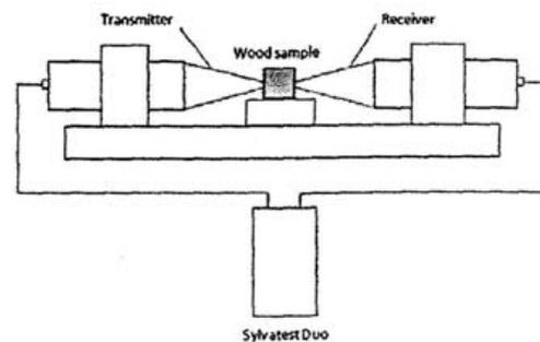
**Figure 3.- Ultrasonic transmission test on small samples.**
