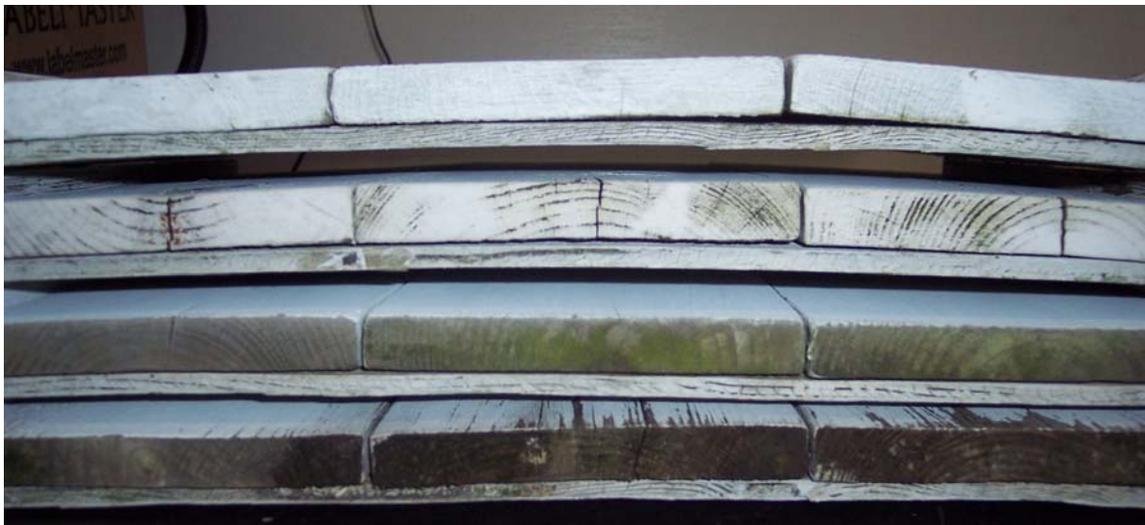
**Figure 11: Drip edge of SYP boards at 12 years. From top: +paint+CuN, +paint-CuN, -paint+CuN, -paint-CuN. Note dark fruiting bodies pushing through paint from latewood of second board.**
