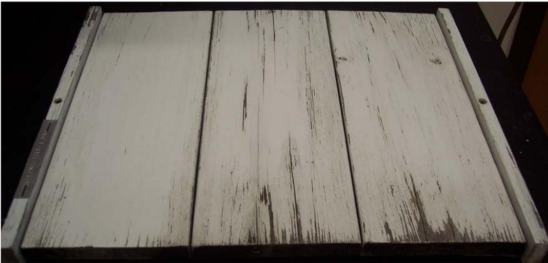
Figure 1: Layout of vertical siding specimens+ ratings at 12 years. Top: SYP, unpainted drip edge+CuN. Substrate (L to R) 8,9,10: Flake 9,9,9. Bottom: SYP, unpainted drip edge, no CuN. Substrate 9,6,7: Flake 8,7,7
