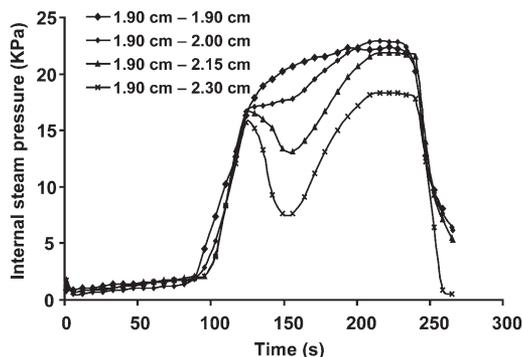
Figure 6. — Effect of burp opening position on the internal steam pressure for 56- by 56-cm panel.
