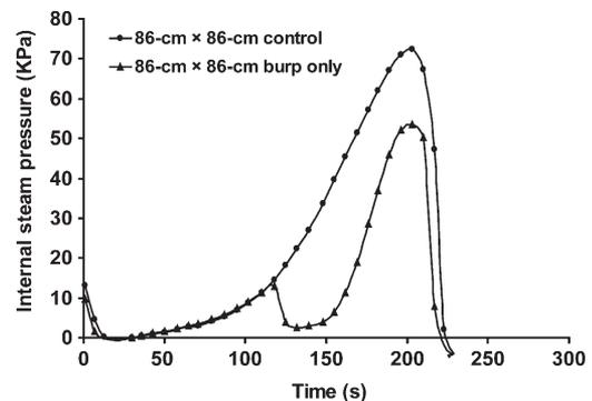
Figure 7. — Effect of burp-opening position on the internal steam pressure for 86- by 86-cm panel.
