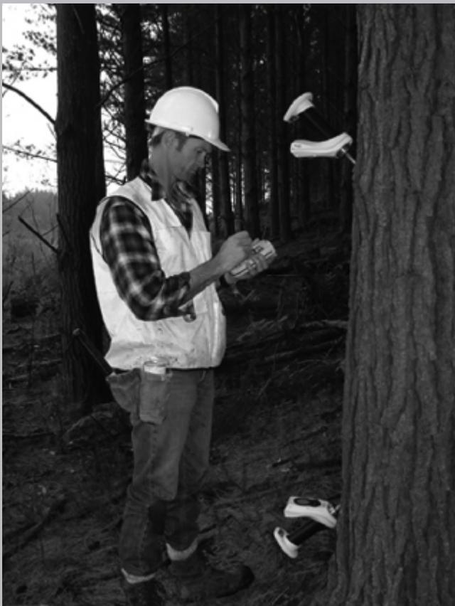
Figure 3. — Application of acoustic tomography in tree decay detection in an urban environment.
