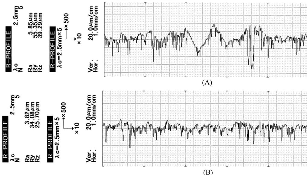
FIGURE 1.—Typical surface roughness profiles of control panel (A) and panel treated at 225°C for 30 min (B).
