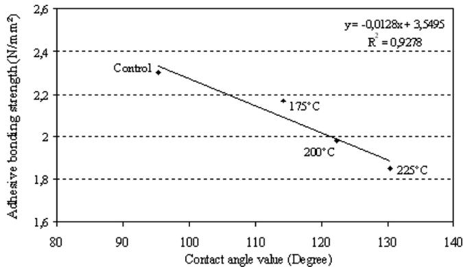
FIGURE 2.—Linear relationship between adhesive bonding strength (delamination of the UF resin bondline between MDF-panel surface and a sheet of beech veneer) and contact angle values.
