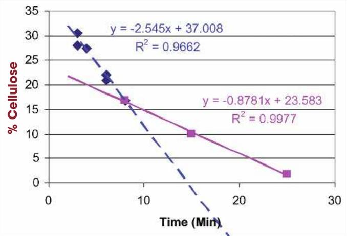
Figure 4. — Relative conversion efficiencies of amorphous cellulose (blue) and crystalline cellulose (red) (derived from: Harris et al. 1985).
