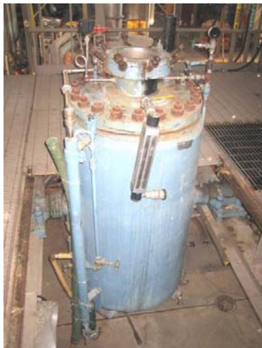
**Figure 1:** The 300-liter or 50 kilogram (dry weight basis) laboratory-capacity digester used to pre-treat red pine (*Pinus resinosa*) with the OA and DEO solutions or with a hot-water (control) cook prior to pressurized steam refining.
