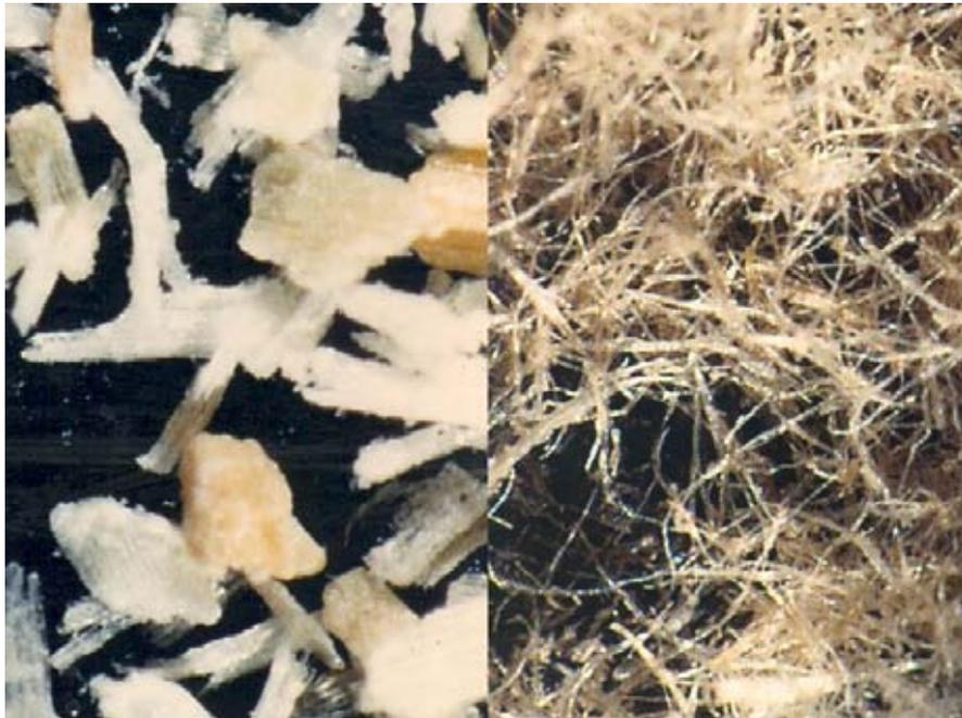
**Figure 3:** Comparison of commercial 40-mesh mixed pine wood flour (left) and processed and refined pine fiber passed through a 40-mesh screen (right).
