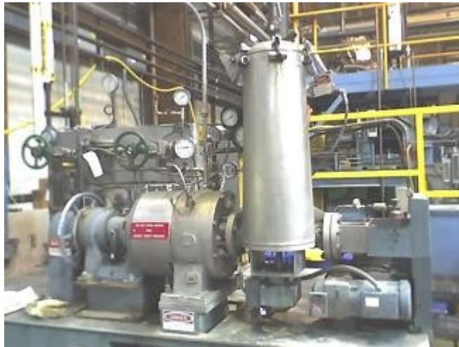
**Figure 2:** The pressurized 300-mm thermomechanical refiner used in this study to make wood fiber
