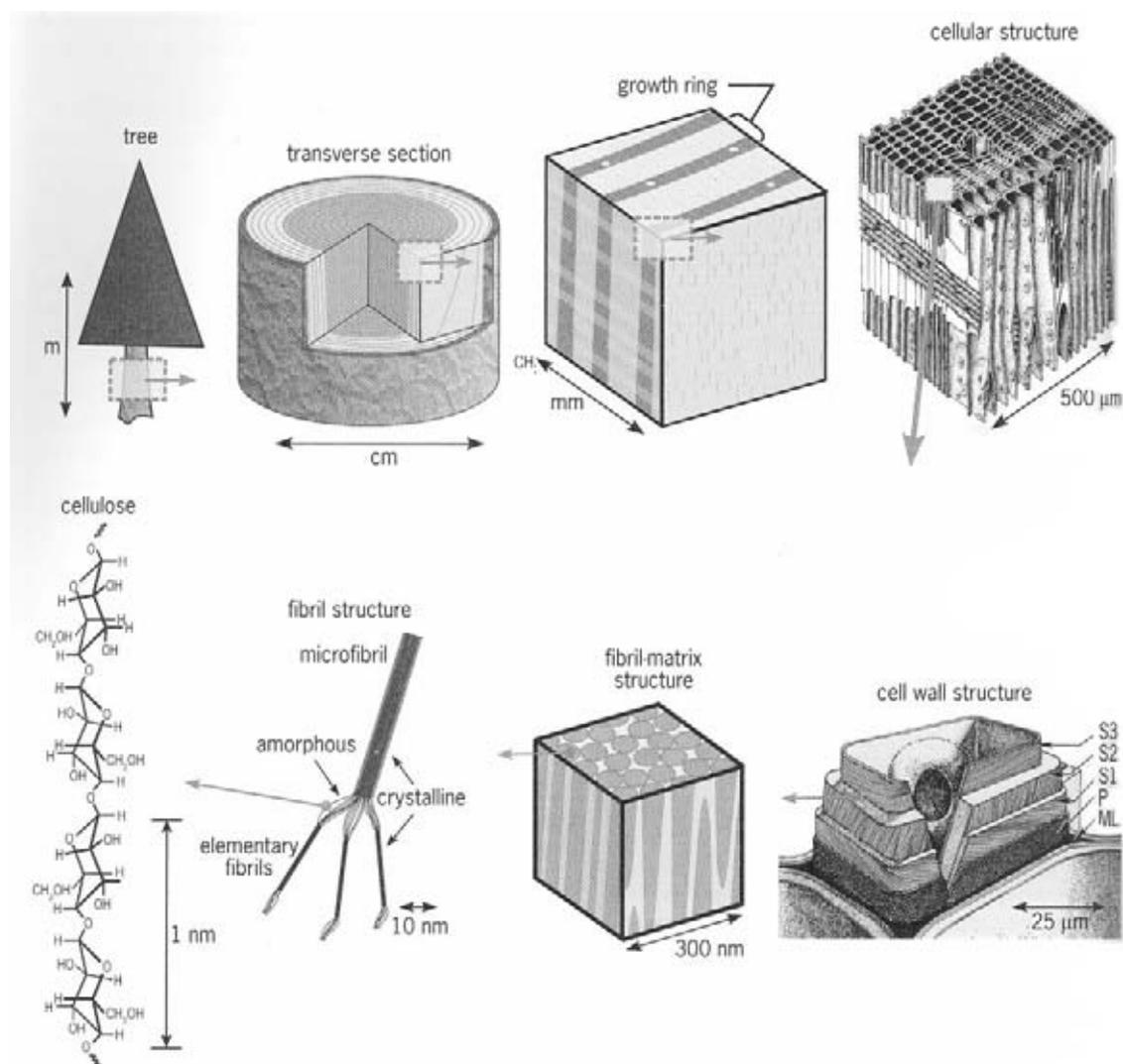
**Fig. 1.** Hierarchical structure of wood, showing the size scale of each structural feature within wood. The linear polymer chains of cellulose (30% of wood by weight) arrange to form cellulose fibrils, which are the base strengthening component within wood. (Adapted from R. J. Moon, C. R. Frihart, and T. Wegner, *Nanotechnology applications in the forest products industry*, *Forest Prod. J.*, 56(5):4–10, 2006)
