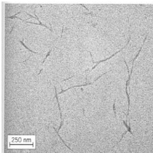
Fig. 2. Transmission electron microscope image of a cellulose nanocrystal. (Courtesy of James Beecher, USDA Forest Service, Forest Products Laboratory, Madison, Wisconsin)
