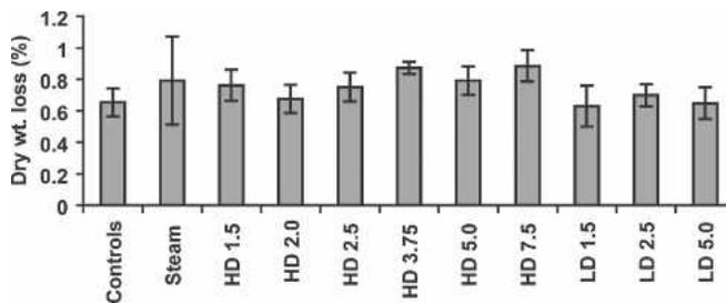
Figure 1. — Comparisons of oven-dry mass loss caused by steam/irradiation, with each vertical bar indicating  $\pm 1$  SD from mean weight loss value. Groups are indicated as the high dose (HD) rate of 1.69 Mrad/h or low dose (LD) rate of 0.85 Mrad/h, with the total dose indicated from 1.50 to 5.0 Mrad.
