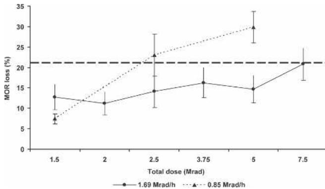
Figure 2. — Relationship between strength loss and irradiation dose, with each vertical bar indicating  $\pm 1$  SD from mean MOR value. For comparison, the mean effect of steam sterilization is indicated by the dashed line.
