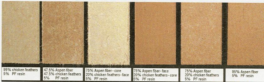
FIGURE 2. Pre-pressed mats: (a) single-layer mat showing uniform distribution of aspen fiber; (b) triple-layer mat with aspen fiber on faces and CFF in core
