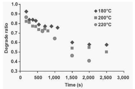
Fig. 5. Effects of press temperature and duration on arabinan content relative to controls.
