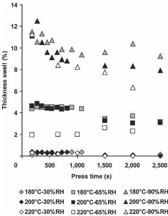
Fig. 3. Relationship between thickness swell at 27°C and RH levels of 30, 65, or 90% for 12.5-mm-thick MDF as affected by press temperature and duration.
