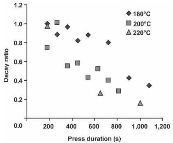
Fig. 4. Comparative decay ratio for non-ground-contact decay of 25- by 25- by 12.5-mm-thick MDF blocks assessed using the Micales-Glaeser (2006) petri dish method. A decay ratio of 1.0 represents the ~20% weight loss experienced by MDF controls.
