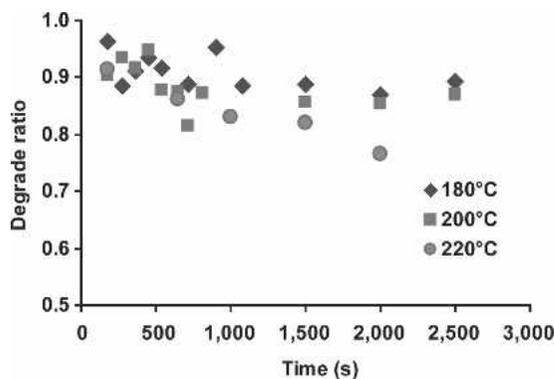
FIG. 7. Effects of press temperature and duration on mannan content relative to controls.
