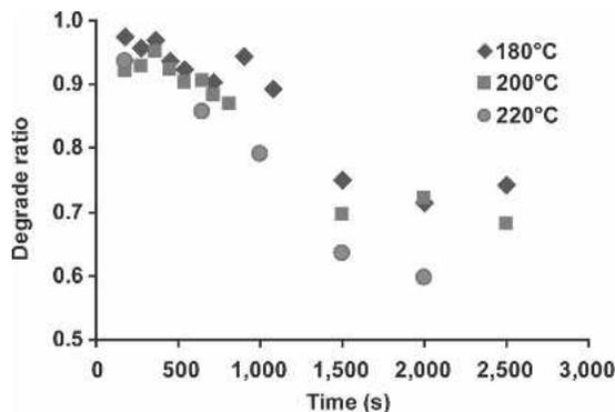
FIG. 6. Effects of press temperature and duration on galactan content relative to controls.
