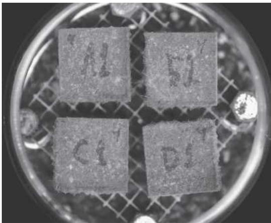
FIG. 1. Example of four non-ground-contact decay tests well underway using the 100-mm petri dish method of Micales-Glaeser (2006).
