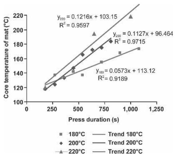
FIG. 2. Effects of press temperature and duration on mat temperature and simple linear estimates of trends.
