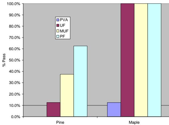
Figure 3. The three-cycle soak/dry tests using pine and maple bonded with PVA, UF, MUF, and MF adhesives determined the percentage of samples that passed the delamination test ( $n = 8$ ).
