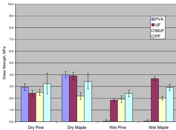
Figure 4. Lap shear tests using PS-1-95 on maple and pine bonded with PVA, UF, MUF, and PF adhesives ( $n = 6$ ).
