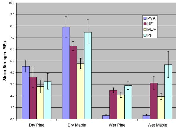
Figure 2. ABES/Instron data for pine and maple lap shear specimens bonded with different adhesives ( $n = 5$ ).
