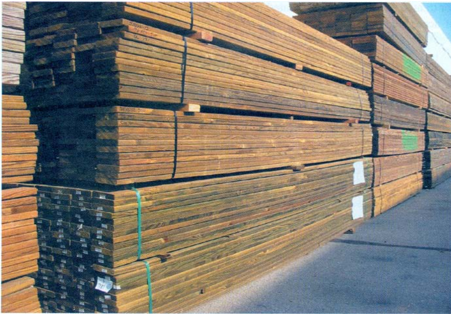
An end tag is used to reveal if wood has been treated to standard specifications.
